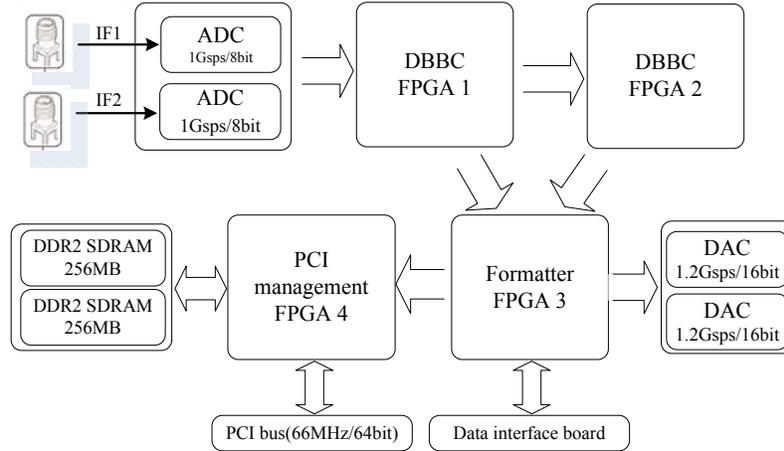
**Figure 3. Signal acquisition and processing board configuration**
