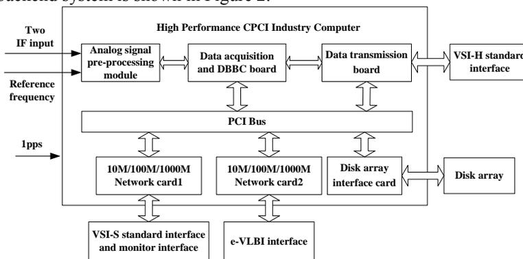
**Figure 2. Deep space interferometry digital backend system configuration**
