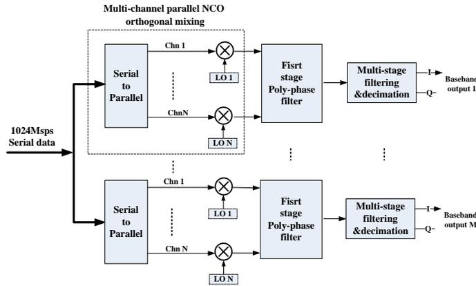
Figure 5. Block diagram of complex data stream output scheme
