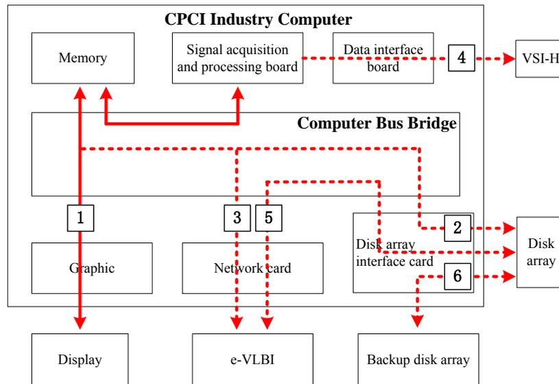
**Figure 6. The schematic diagram of the data transmission and recording**
