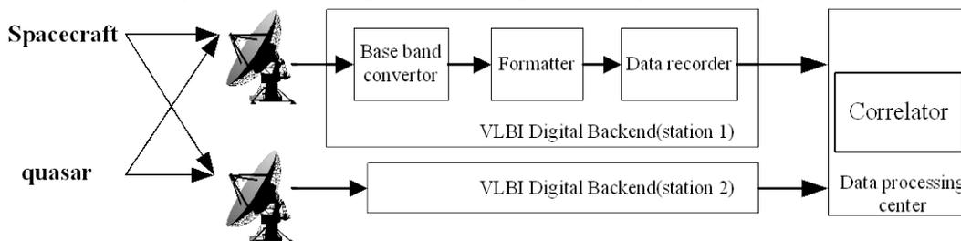
Figure 1. The structure and signal processing flow of Delta-DOR
