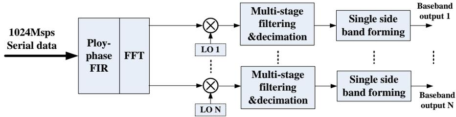
Figure 4. Block diagram of real data stream output scheme
