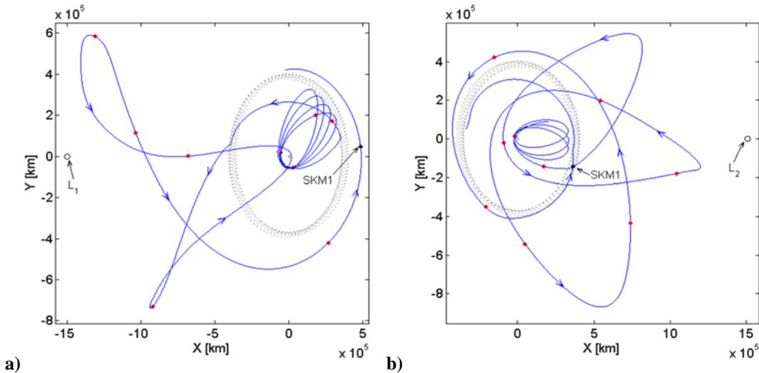
**Figure 4. The definitive Trans-Lunar trajectories in a Sun-Earth rotating frame, with the Sun in the negative X direction. The DSMs and TCMs are marked in red. SKM1 marks the start of the Libration Orbit phase. The Sun-Earth libration points are labeled as L1 and L2 respectively. The dotted trajectory shows the Moon's orbit during this time period. a) P1 b) P2**
