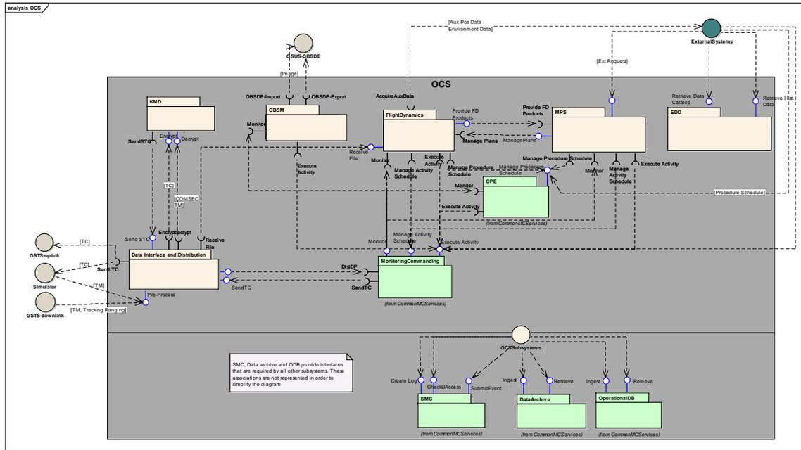
Figure 2 Operational Control System Architecture Featuring Common Components and Interfaces
