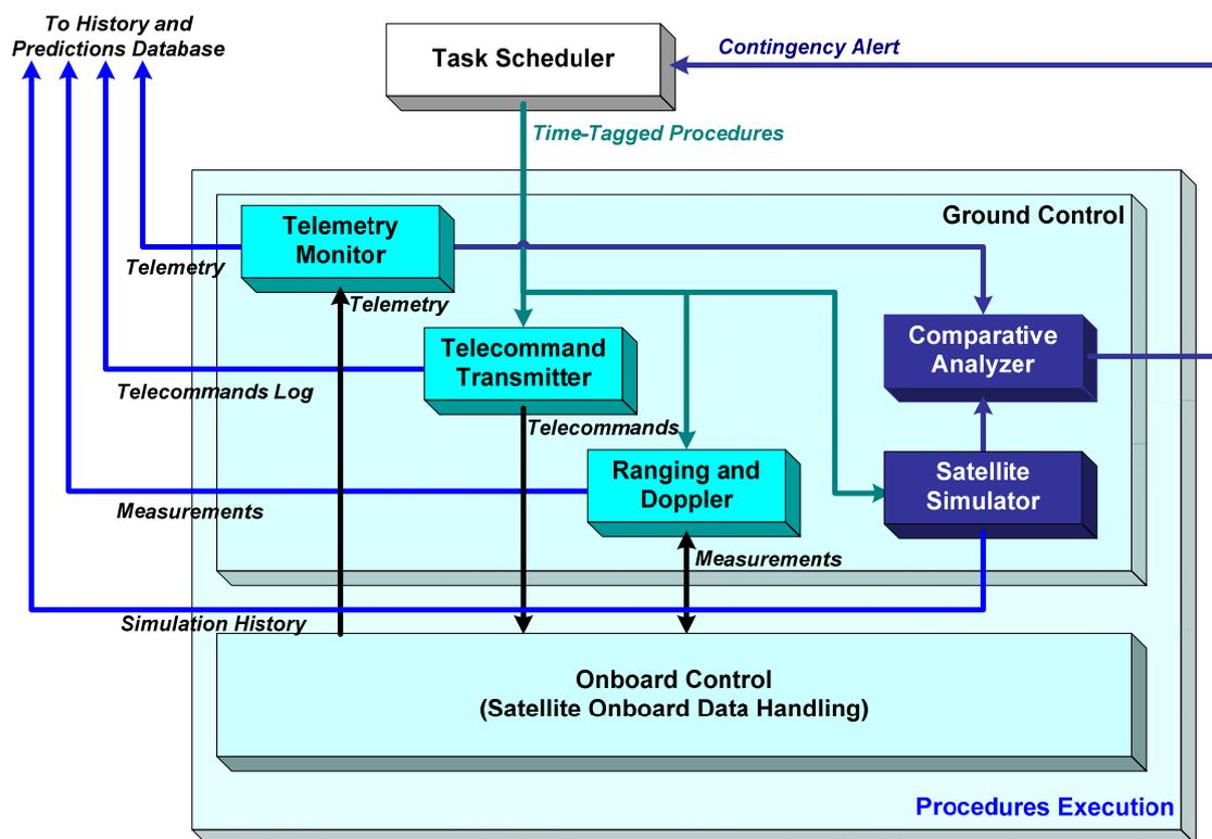
Figure 4. Newly Proposed Procedures Execution Subsystem Architecture
