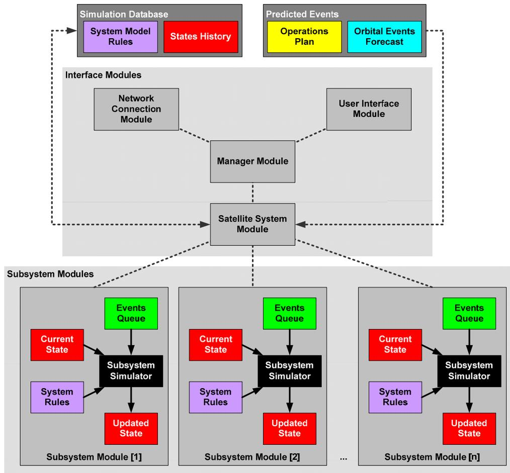
**Figure 8. Planning Verification Satellite Simulator Architecture**
