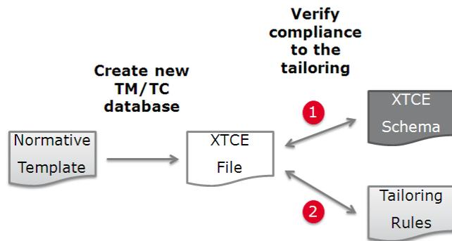
**Figure 6. Tailoring Usage Scenario.** A new TM/TC database is created from the normative template, and needs to be checked first against the XTCE schema and then against the tailoring rules.
