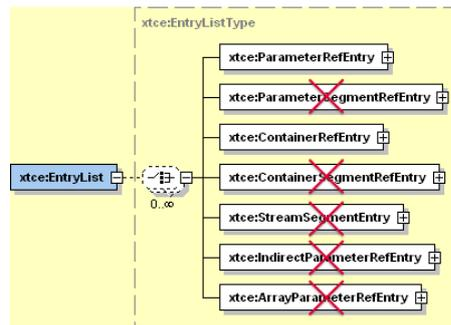
**Figure 3. Tailoring Example.** From seven supported ways to define a packet entry in XTCE, only two are allowed.
