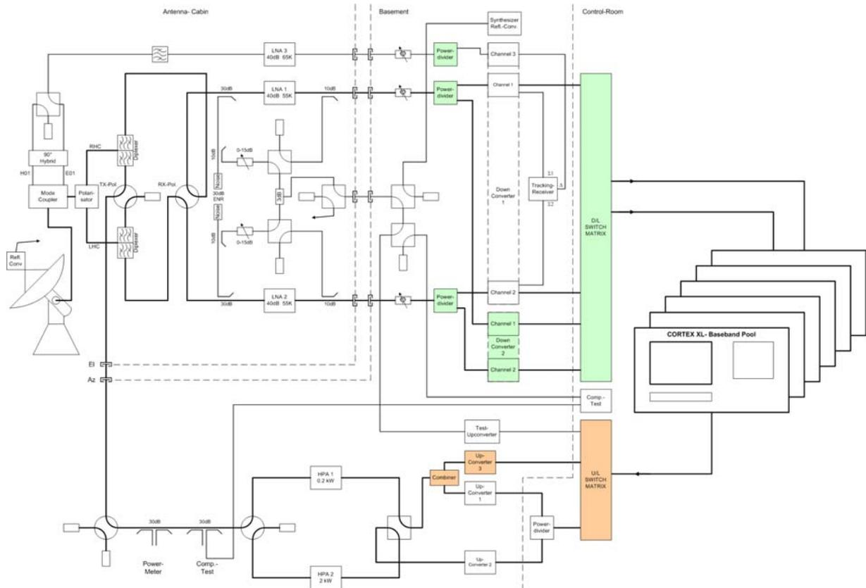
Figure 2. The new block diagram of the 15-meter S-Band antenna.
