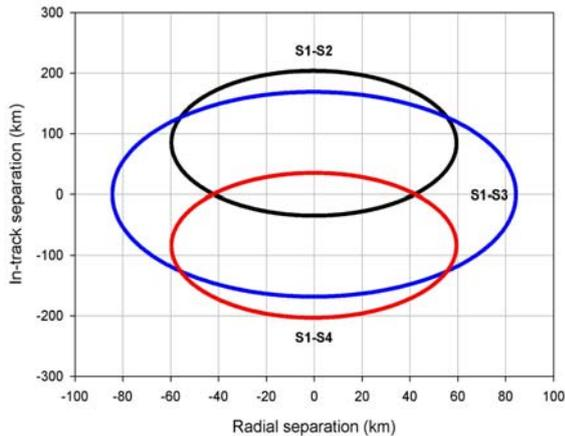
Figure 5. Radial and in-track separation of IGSOs.
