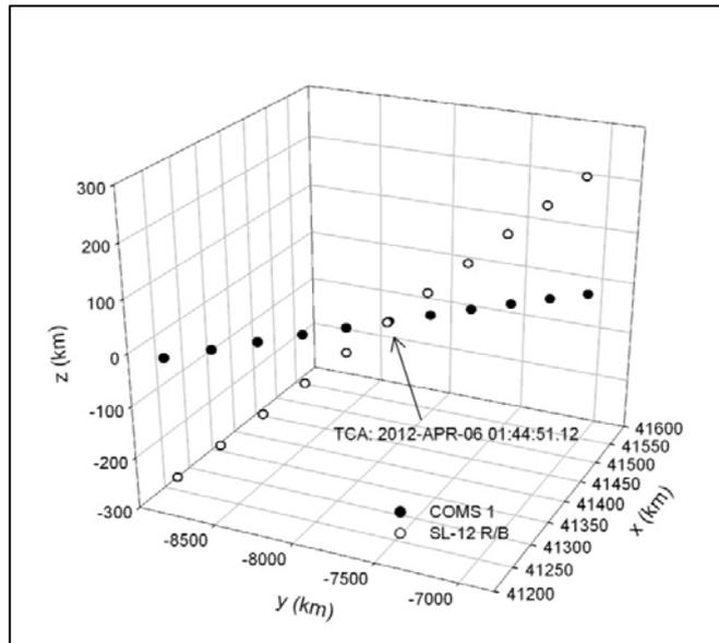
Figure 14. 3-D positions of two satellites near TCA.
