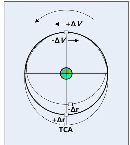
Figure 15. Effect of  $\Delta V$  operation.
