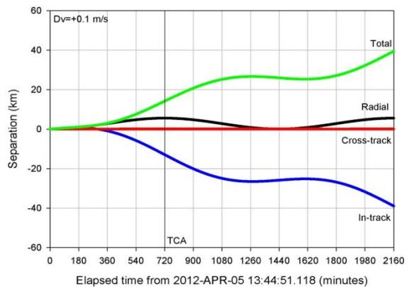
**Figure 16. Separation of COMS1 with and without CAM.**
