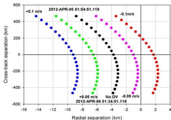
**Figure 17. Radial and in-track separation near TCA. Figure 18. Radial and cross-track separation near TCA.**
