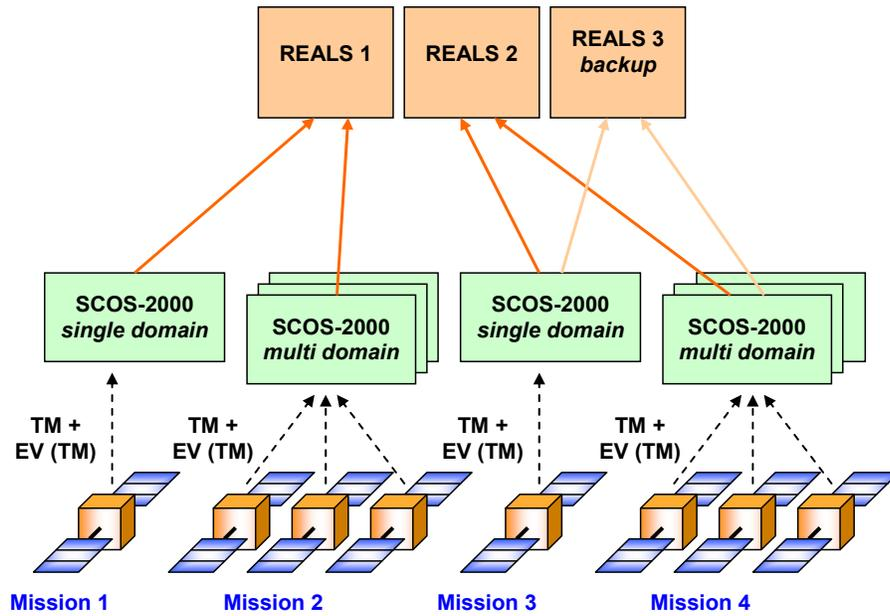
Figure 2. REALS multi-mission, multi-domain, and redundancy.
