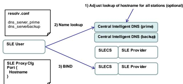
The figure above shows the basic architecture, which can easily be extended for external users. At any point in time the ESTRACK operators can adjust the name resolution for the prime and backup chain. When an SLE connection is established, the hostname is looked up via the ‘Intelligent DNS’ and the SLE connections are established to the correct prime and backup chains.
