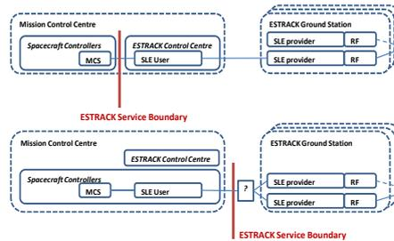
Therefore, the operator of the SLE User shall, via voice communication, confirm with the ECC Operator the prime chain for the pass, and use the set of SLE Service Instances (SI) corresponding to that particular communication chain in the ground station. Similarly, error-handling requires coordinated manual intervention between the two entities responsible for the operations of SLE User and SLE Provider to ensure SLE links are consistently re-routed.
