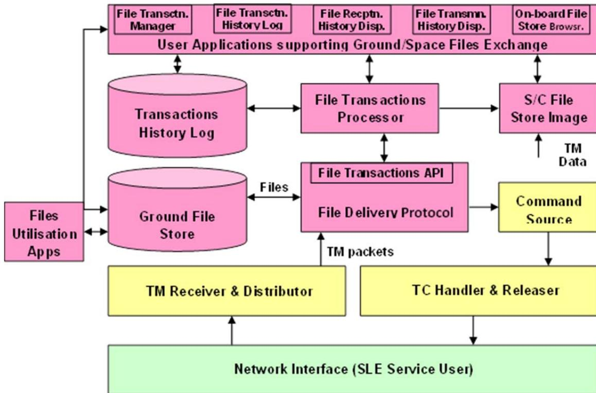
**Figure 4. High-level architecture of the Control System components supporting File based Operations**
