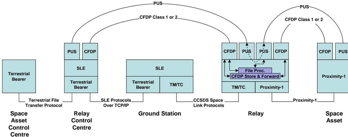
**Figure 3. Proposed solution for file based Space Asset Control operations via a Relay in space.**
