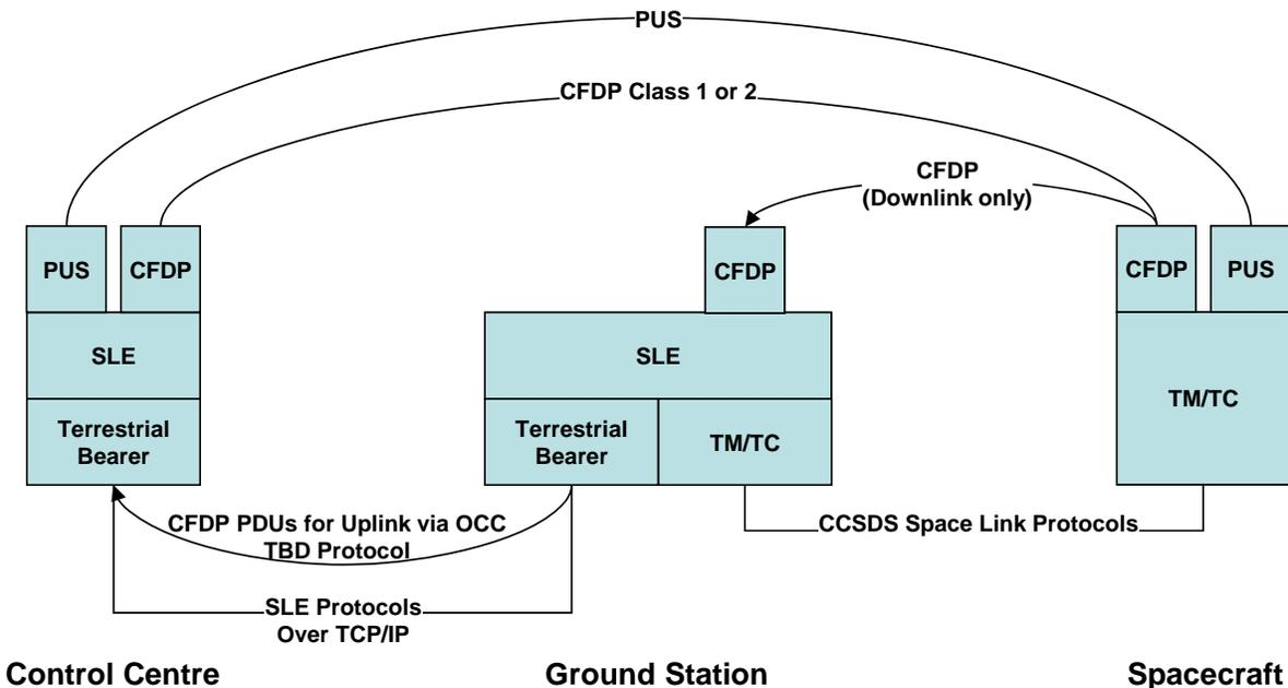
**Figure 2. Proposed solution for file based Spacecraft Control operations. File Delivery to ground station.**
