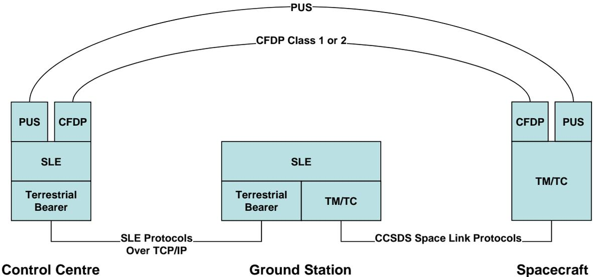
Figure 1. Proposed solution for file based Spacecraft Control operations
