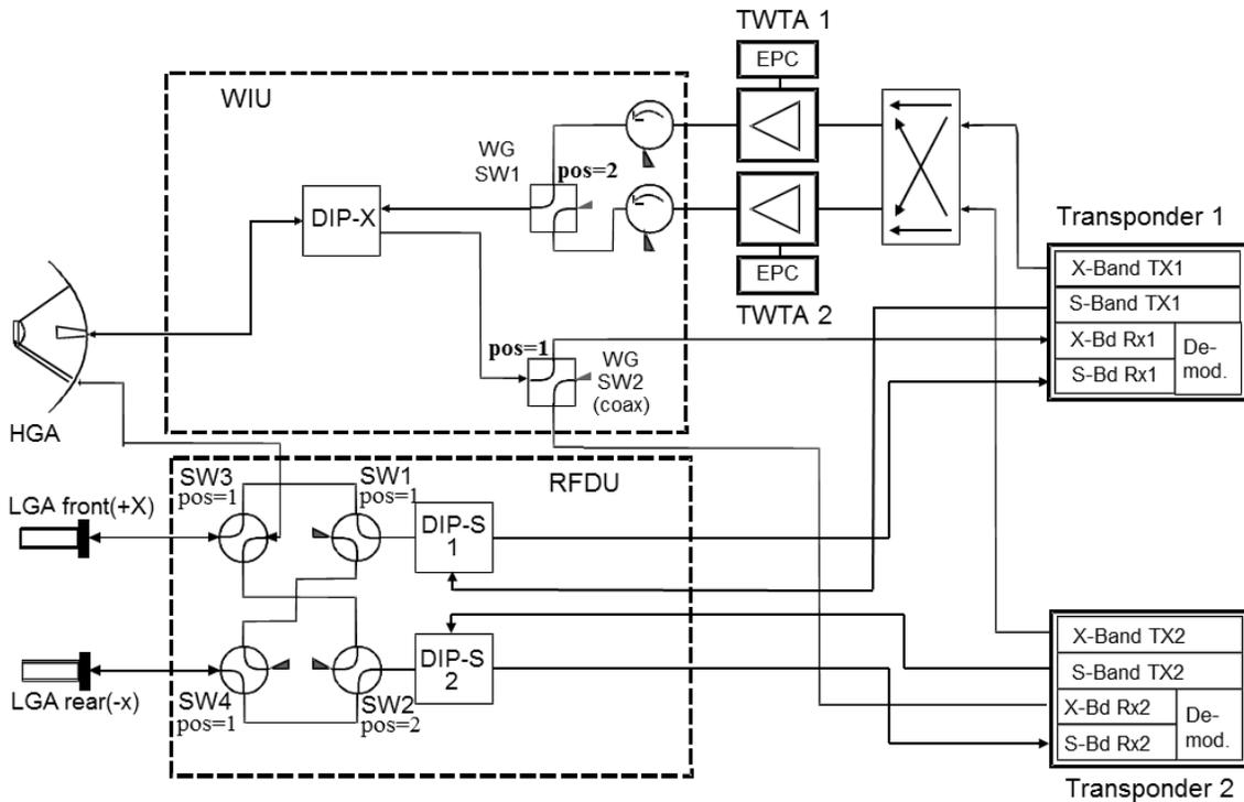
Figure 1. Block Diagram of Mars Express TT&C System
