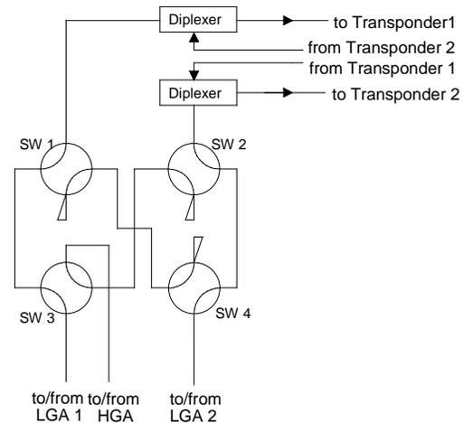
Figure 3. Mars Express RFDU Block Diagram
