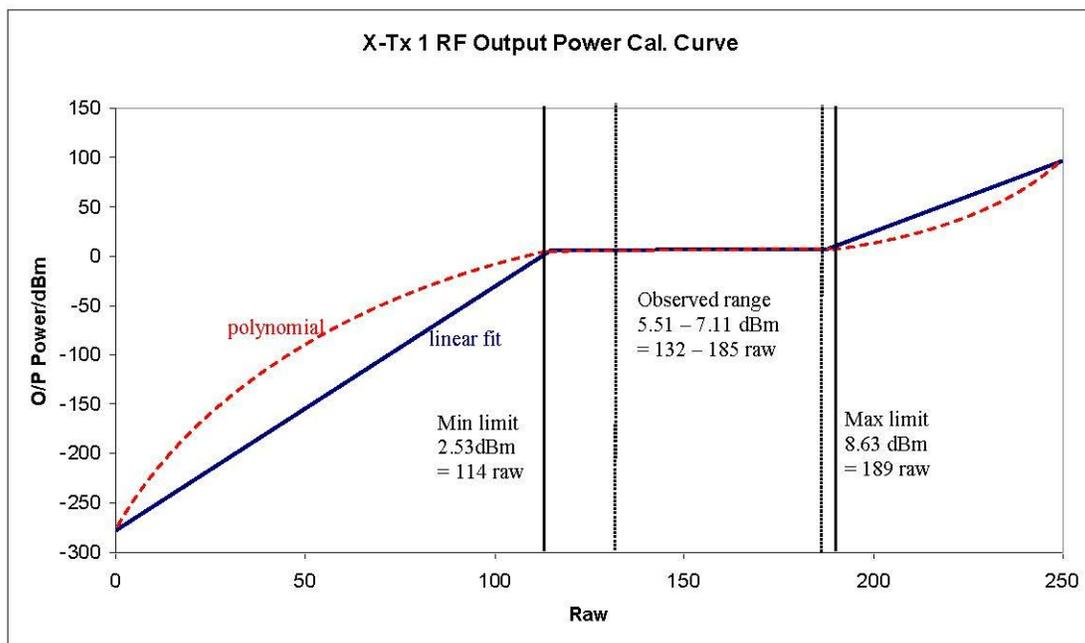
Figure 4. X-Tx-1 Output Power Calibration Curve and Limits
