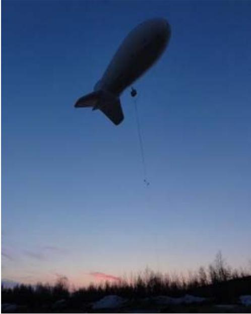
**Figure 6. Ascending Blimp with microphones**
