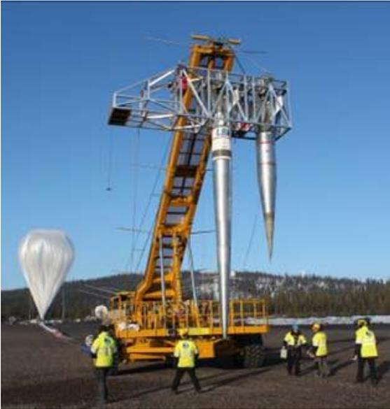
**Figure 5. D-SEND#1 gondola with two drop bodies**
