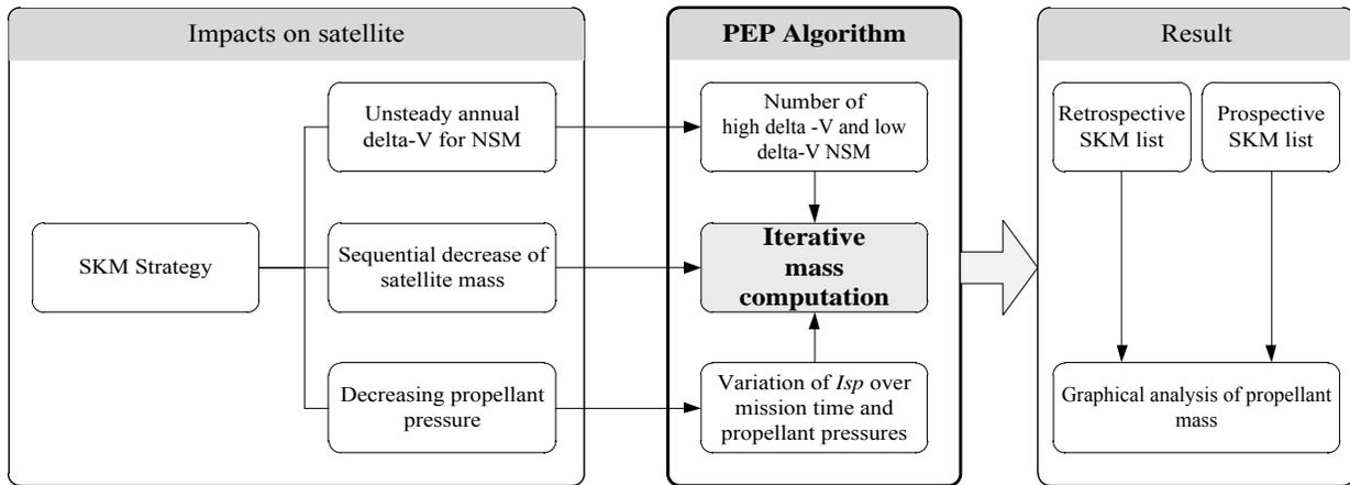
**Figure 3. Processes related to the PEP split into three main groups. Each impact on the satellite leads to a specific computational algorithm. The prospective SKM lists, together with the retrospective SKM list from the mass log, allow a graphical analysis of the propellant mass.**
