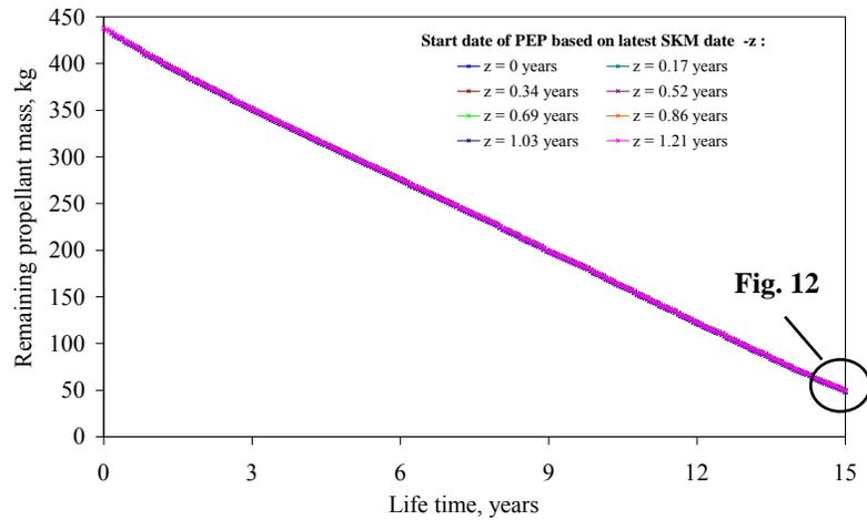
**Figure 11. Propellant mass as graphical analysis from PEP data drawn over the lifetime. Eight different start dates were used to create data with the PEP over 560 iteration steps.**
