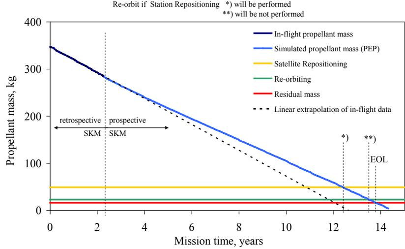
**Figure 4. Graphical analysis as output of the PEP. It shows the curve of remaining propellant mass and its mass boundaries.**
