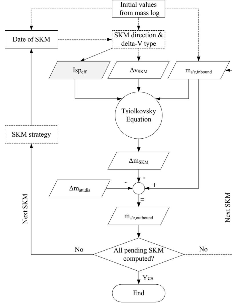
**Figure 5. Process flow of the iterative mass computation as centerpiece of the PEP. The time dependent effective  $Isp$  is not illustrated and is separately explained in IV.B.**
