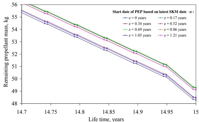
**Figure 12. Propellant mass as output of the PEP plotted over the lifetime zoomed in to EOL.**
