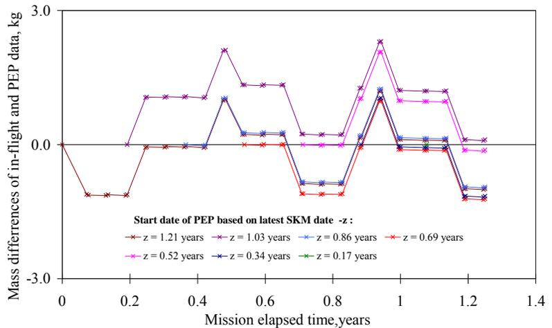
**Figure 10.** Differences between the propellant masses of PEP and in-flight data. The PEP data is based on seven different start dates.
