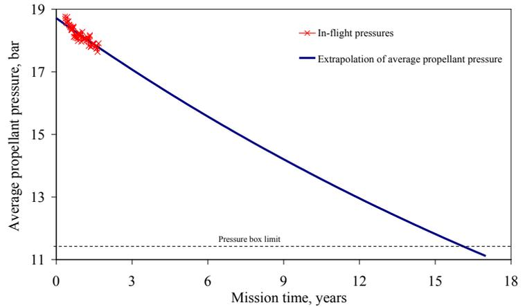
**Figure 7. Exponential extrapolation of propellant pressures based on in-flight data.**
