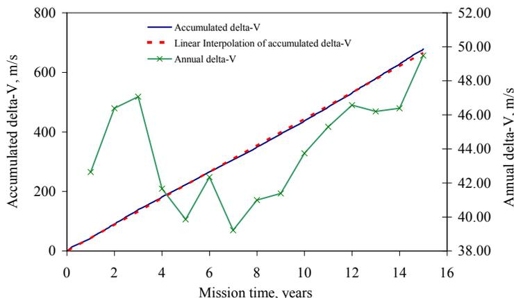
**Figure 2. Accumulated delta-V compared with the annual delta-V. The variation of the accumulated delta-V is visible in comparison to the linear interpolation of the accumulated delta-V.**
