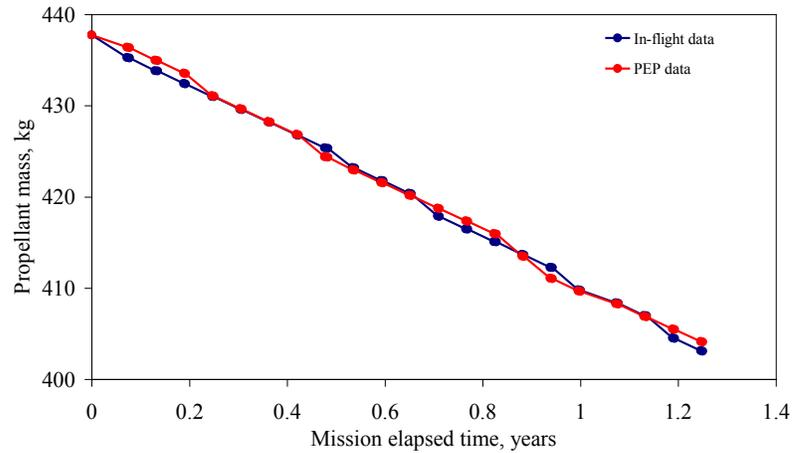
**Figure 9.** The total propellant masses from the PEP and in-flight data show the consistency of the PEP with small aberrations.
