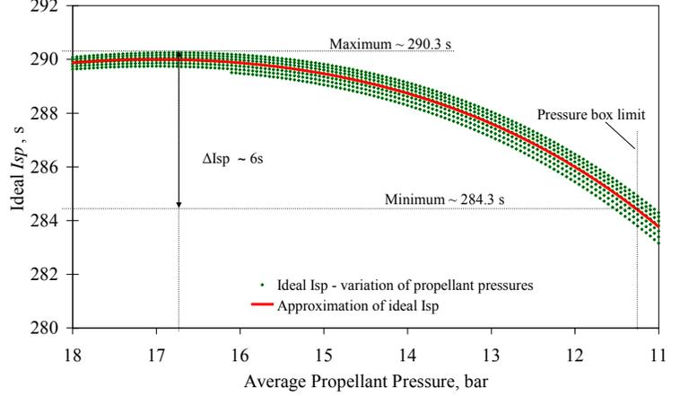
**Figure 8. Polynomial approximation curve of ideal  $Isp$ . Derived by calculating the  $Isp$  with varying propellant pressures as input.**
