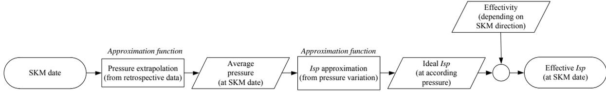
**Figure 6. Process of transforming a maneuver time into the effective  $I_{sp}$ . The ideal  $I_{sp}$  is calculated with the time dependency of the propellant pressures and the pressure dependency of the ideal  $I_{sp}$ .**
