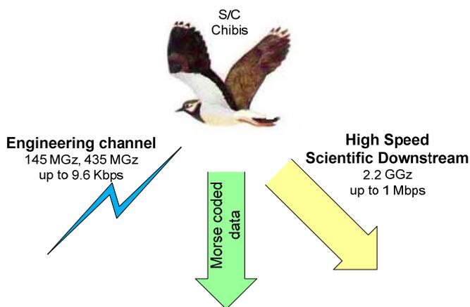
**Figure 2** Up and Down-links in “Chibis-M” mission. (In Russian “Chibis” means lapwing)
