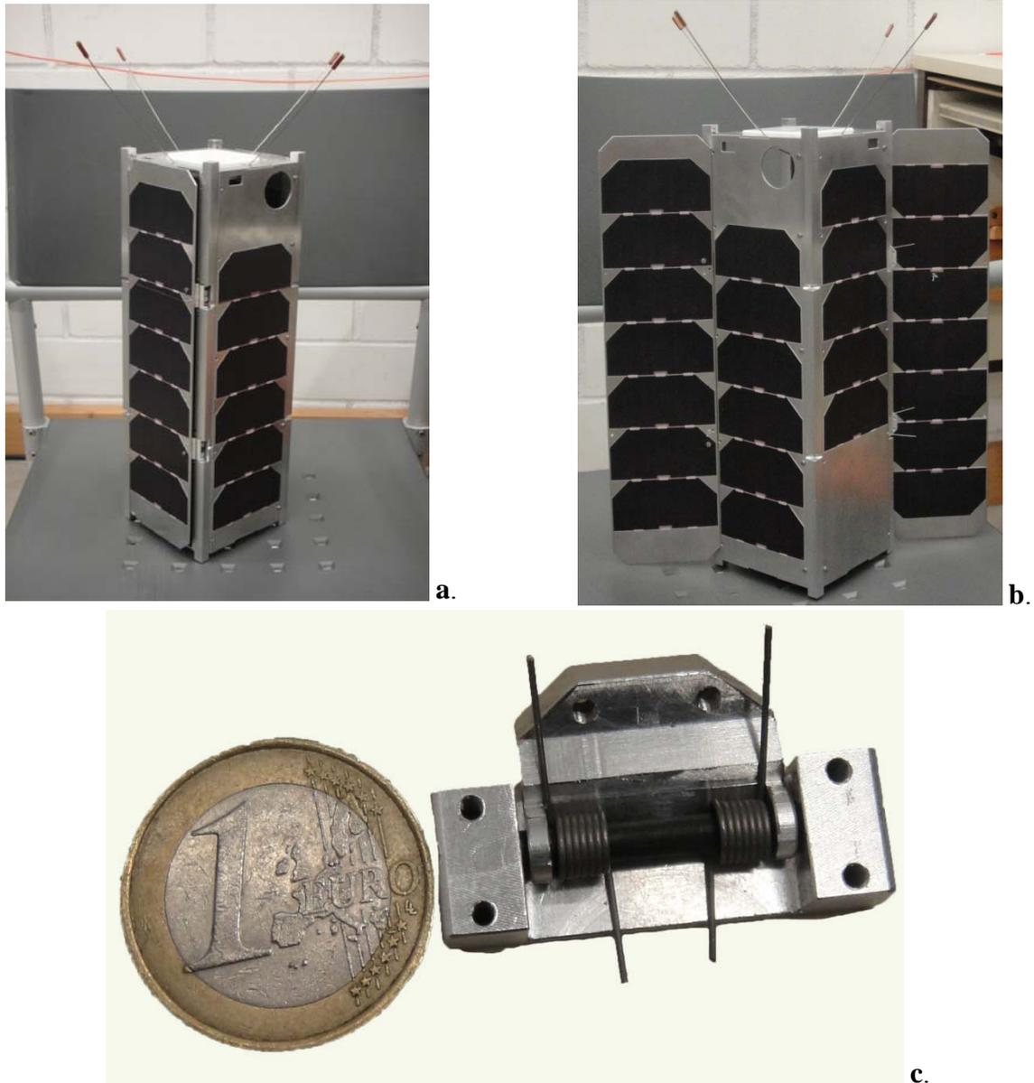
Figure 9 a. Stowed position of the Satellite using fishing line; b. Deployed position of the panels at 135°; c. Assembly of torsion springs, lever, rod and socket
