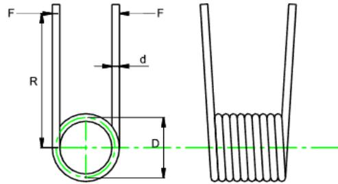
Figure 1 Torsion Spring
