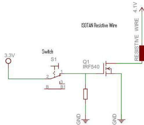
Figure 2 Schematic diagram of release mechanism
