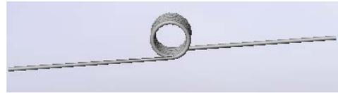
**Figure 6 CAD of Torsion Spring**
