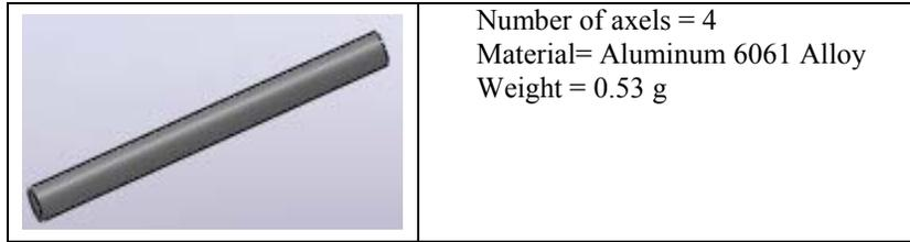
Figure 7 Different parts of the deployment mechanism
