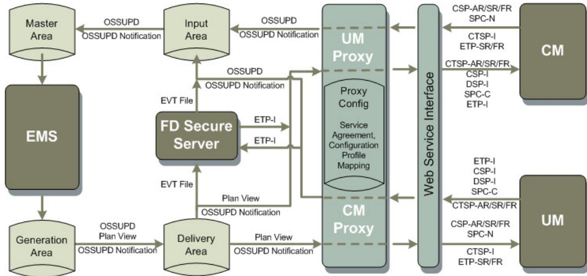
**Figure V-1 High Level Architecture of the SCCS-SM Proxy in EPS/ESS<sup>5</sup>**
