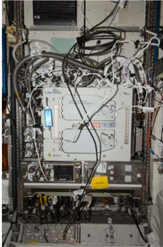
Figure 1. EMCS on orbit, integrated into EXPRESS Rack 3 inside the Columbus module.
