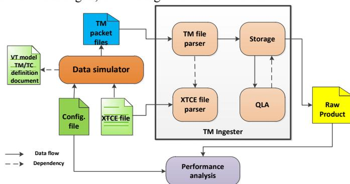
Figure 2. Basic architecture and data flow of the TM ingester.
