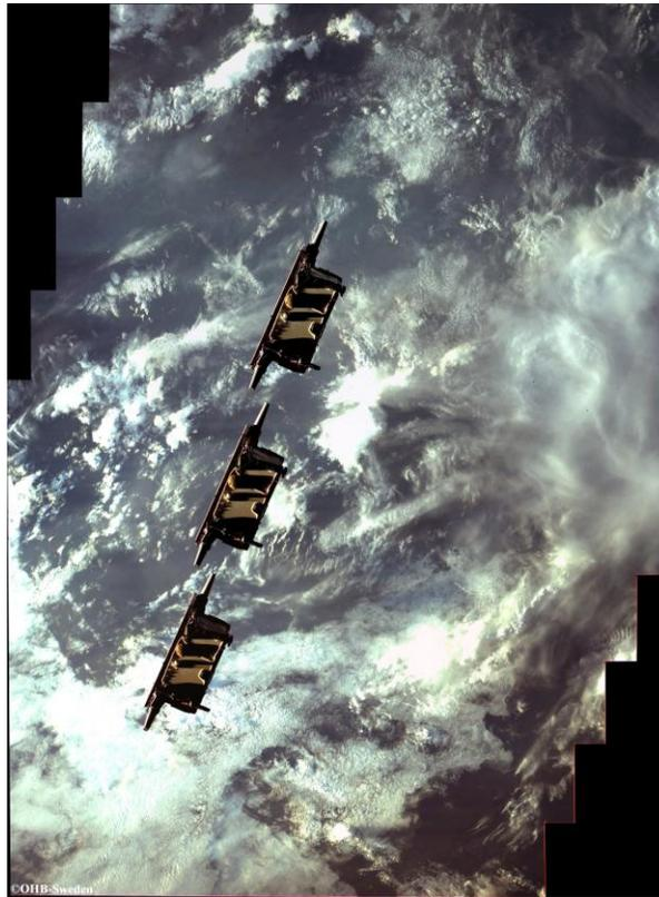
**Figure 4: Tango spacecraft captured from Mango when flying in a controlled nadir formation
