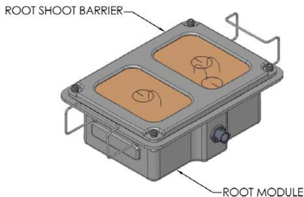
**Figure 2. EPO Greenhouse root module assembly with root shoot barrier**
