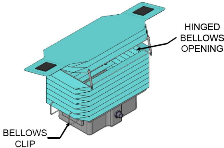
**Figure 1. EPO Greenhouse Growth Chamber showing bellows clip used to set bellows height and hinged bellows opening.**
