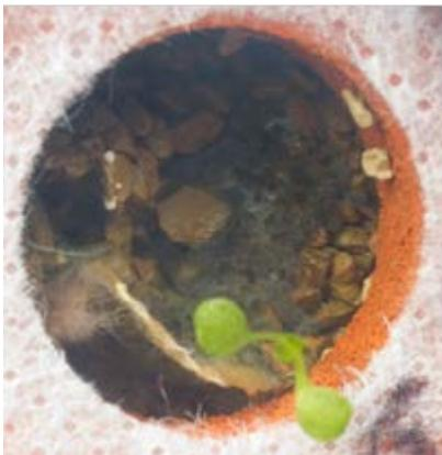
**Figure 10. Growth of Mold confirmed in plug hole**
