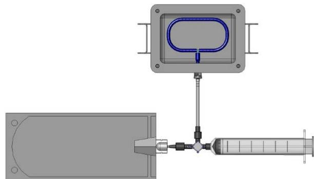
**Figure 3. Syringe attached to water bag and root module assembly (bellows, root shoot barrier and growth medium removed for clarity)**
