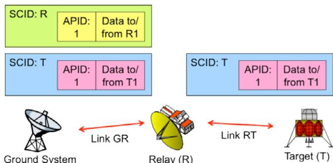
Figure 6. Multiplexing at the Frame level.
