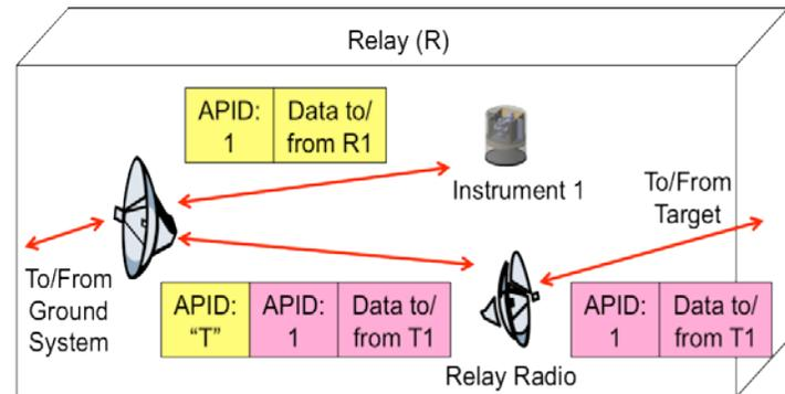
**Figure 8. How Packets are routed in Relay (R).**
