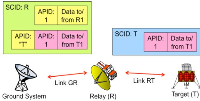
**Figure 7. Multiplexing at the Packet level with Packet encapsulation.**
