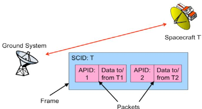
Figure 1. Example of a Frame and Packets used for a single, independent spacecraft.
