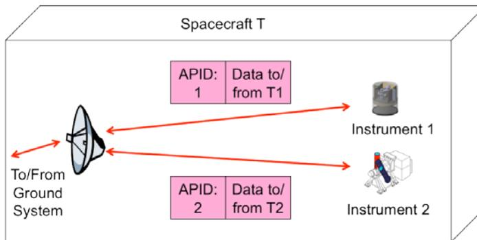
Figure 2. How Packets are routed in a spacecraft.
