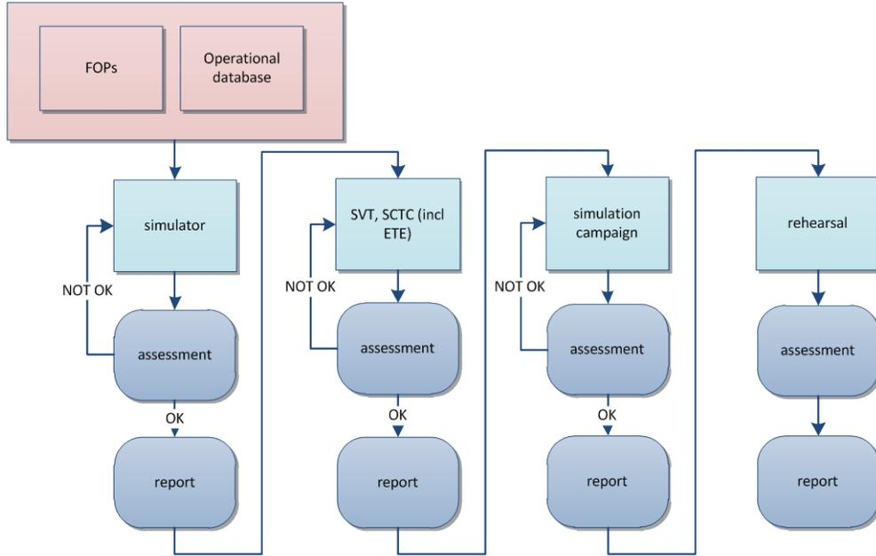
**Figure 4: Operational validation process**
