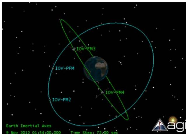
**Figure 1. Predicted 3-dimensional view of the IOV constellation flight for an epoch on November 8, 2012 after completion of the drift manoeuvre for FM3 and FM4**
