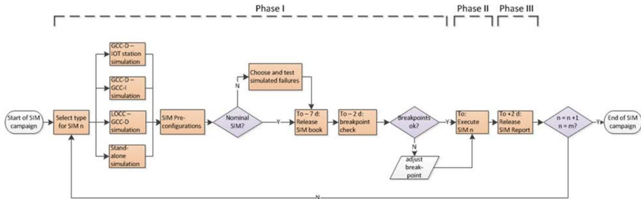
**Figure 4. The applied simulation planning and execution sequence for a stand-alone or multi-control-center simulation  $n$  with its three distinct phases: I – preparations, II – execution and III – follow-up work. The simulation campaign is accomplished when the total number of planned simulations  $m$  is reached.**
