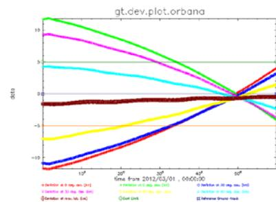
Figure 8. Effect in ground-track evolution of a -15mm/s in-plane maneuver at TCA-6.5 orbits
