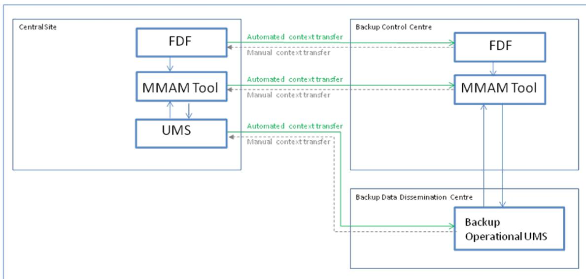
Figure 4 Automatic context transfer between central site and backup centres
