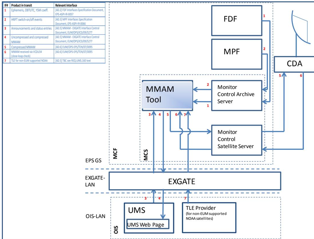
Figure 2 MMAM Functional Elements and Data Flow
