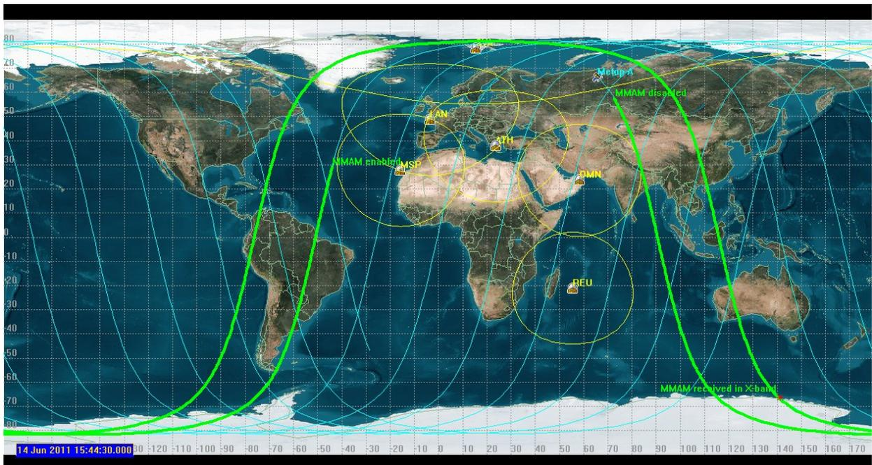
Figure 3 World map showing the Metop-A ground track while downlinking MMAM (green line)
