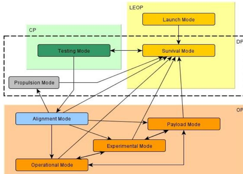
**Figure 2. Operation Modes of the ITASAT-1 spacecraft.**
