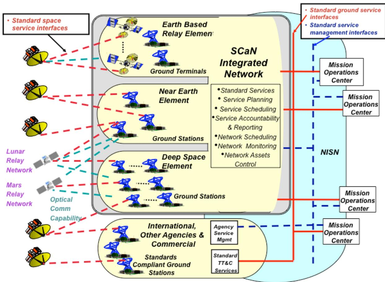
Figure 1: The NASA Integrated Network Architecture in 2018 establishes common user interfaces and enablers for infusion of future technologies
