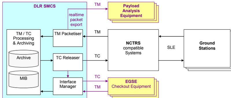
Figure 2. Parallel Support of Groundstation and EGSE interfaces.
