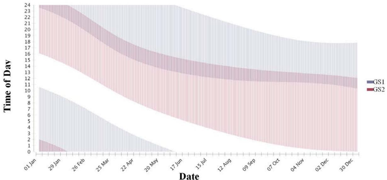
Figure 4. Possible contact periods per spacecraft and ground station
