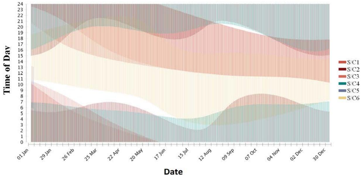
**Figure 5. Possible contact periods per ground station and spacecraft**
