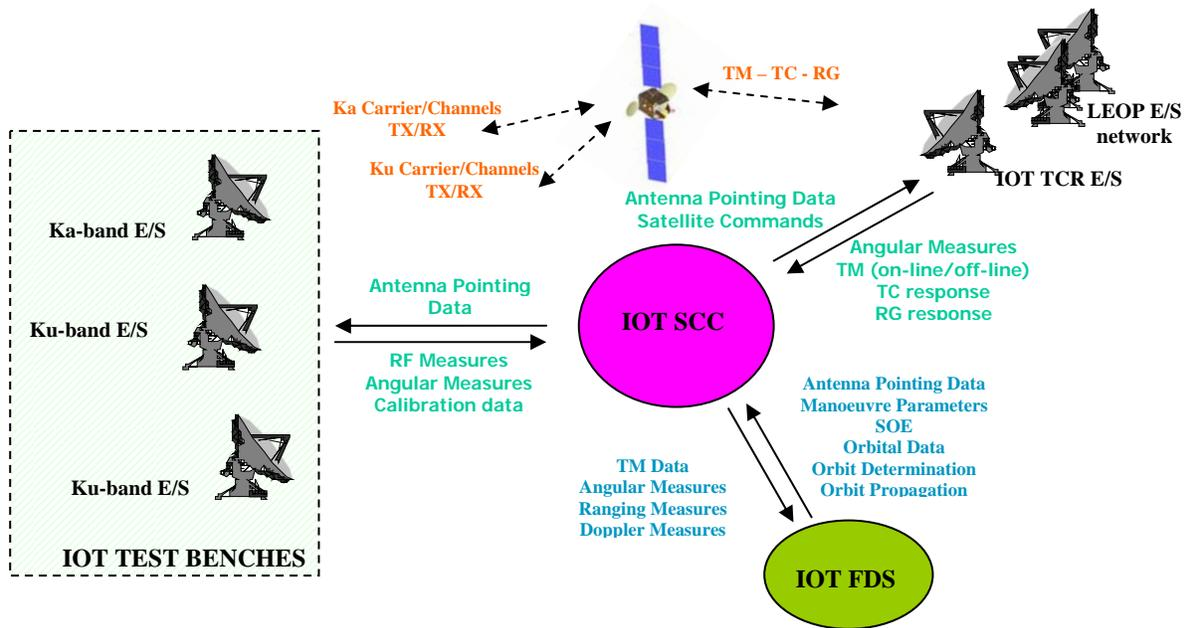
**Figure 2. IOT station schematic.**
