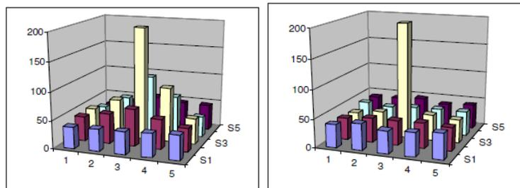
**Figure 10. Examples of a real star (left) and a warm pixel (right) having comparable energy; courtesy of A.Bacchetta.**
