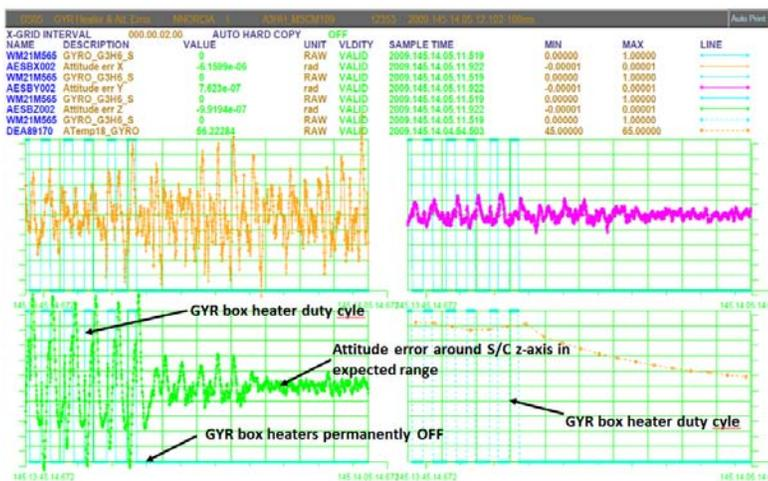
**Figure 7. Plot of the attitude error as seen by the on-board attitude control system at the time when the switching of the external GYR heaters was suppressed.**
