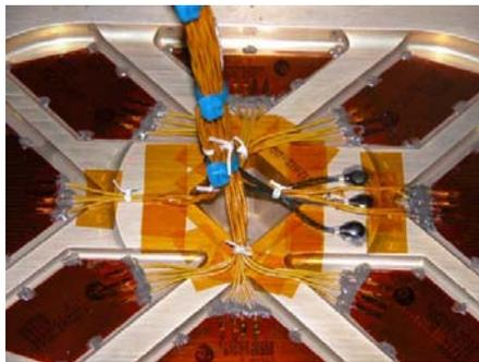
**Figure 6. mounting of the heaters on the GYR base plate**
