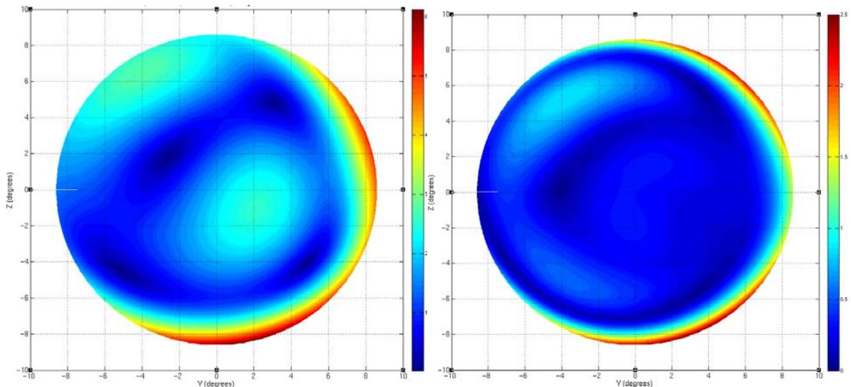
**Figure 15. Residual distortion assessment before and after 3-D update in OD1005; courtesy of M.Tuttlebee.**
