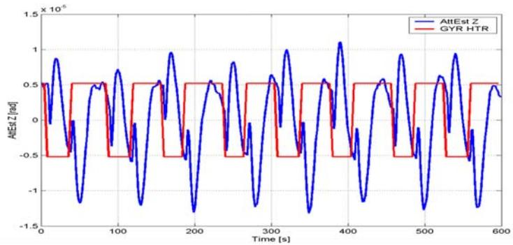
**Figure 5. attitude error around the S/C z-axis overlaid with the duty-cycle of the external heaters attached to the GYR box; courtesy of M.Oort, M.Palomba, Y.Roche**
