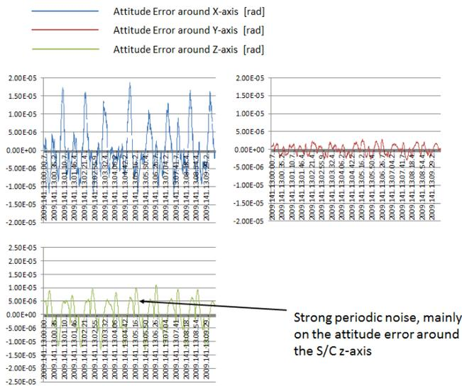
**Figure 4. unexpected noisy attitude error calculation in the on-board attitude control law, violating the Relative Pointing Error specifications**
