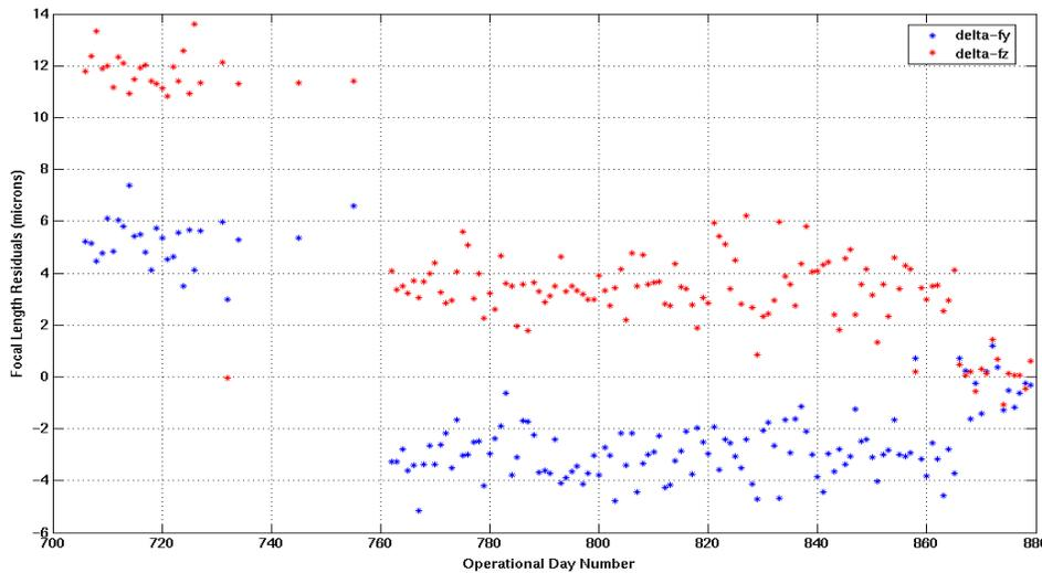
**Figure 14. Evolution of focal length residuals after 1-D update in OD760 and 2-D final update in OD866; courtesy of M.Tuttlebee.**
