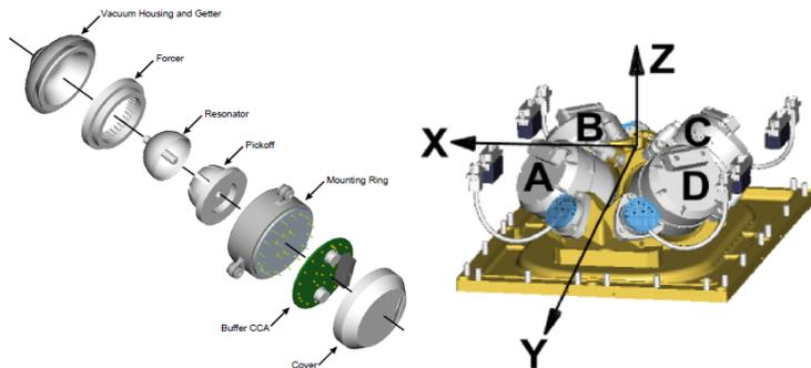
**Figure 3. Hemispherical Resonator Gyro Unit & 4-unit assembly**
