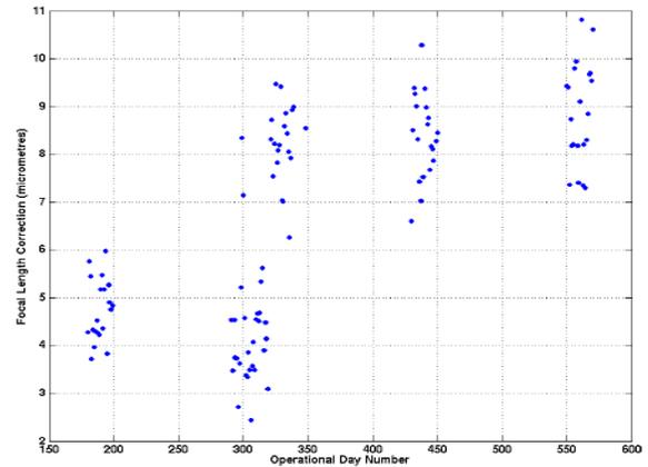
**Figure 11. Estimated Focal Length Correction Evolution; courtesy of M.Tuttlebee.**
