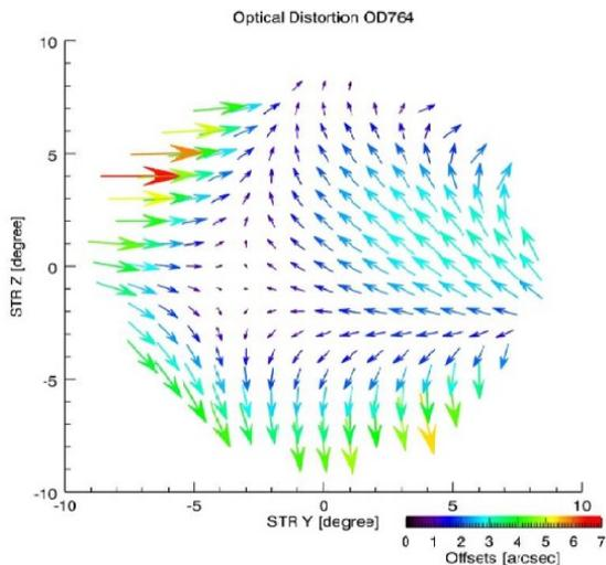
**Figure 12. Residual distortions of the STR1 focal plane, after focal length correction in OD760; courtesy of H.Feuchtgruber.**
