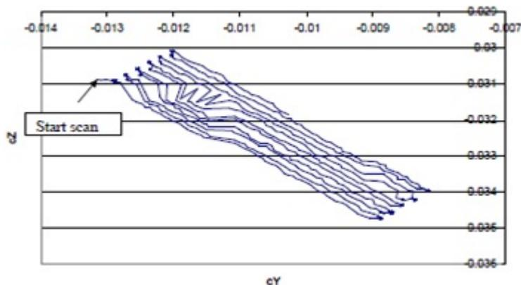
Figure 9. Scan map ‘speed bump’ due to CCD warm pixel; courtesy of M.Oort.
