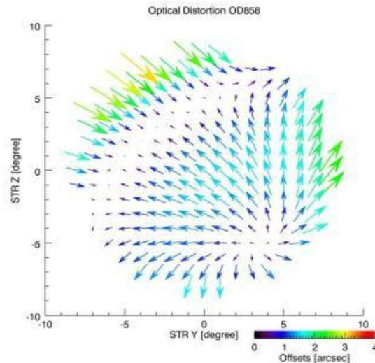
**Figure 13. Residual distortions of the STR1 focal plane, after 2-D distortion coefficient update in OD858; courtesy of H.Feuchtgruber.**
