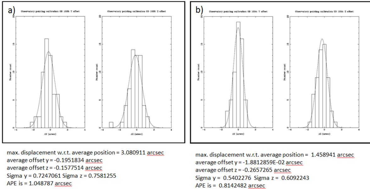
**Figure 17. APE improvement after “star catalogue” clean-up ; a) results obtained prior to clean-up; average APE=1.05 arcsec; b) results obtained after “star catalogue” clean-up; average APE=0.81 arcsec; histograms and figures courtesy of M. Sanchez**
