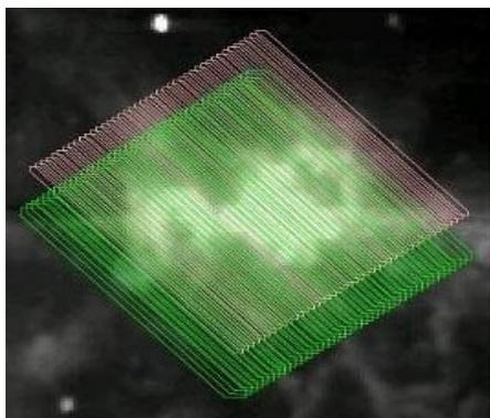
Figure 8. Typical scan map traces by PACS and SPIRE, scanning at ~20"/s
