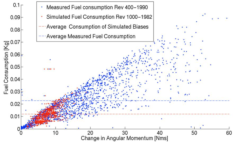
**Figure 7. Comparison between the 3WD fuel consumption and simulated 4WD fuel consumption**
