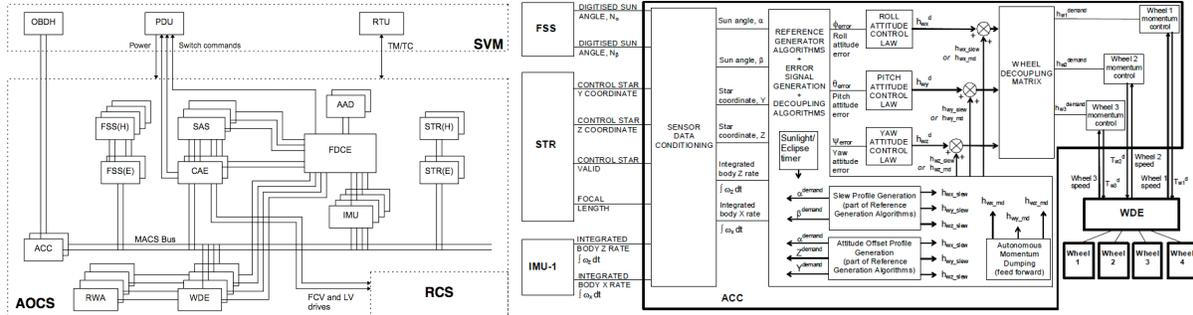
Figure 3. AOCS block diagram (left) and IPS mode logic (right).
