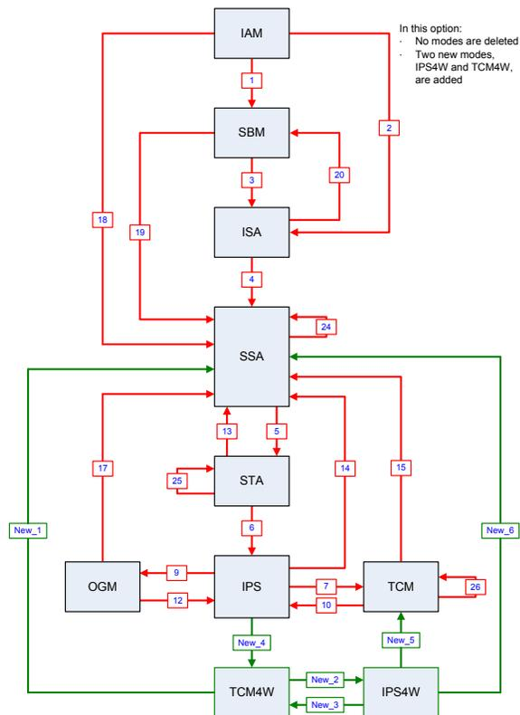
Figure 6. Architecture of the AOCS modes with the new TCM4W and IPS4W for 4WD.
