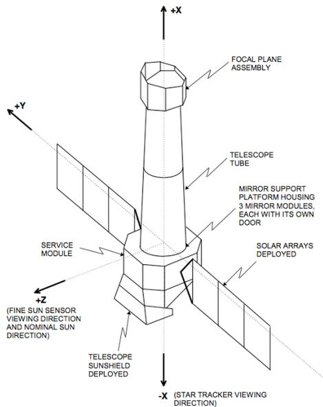
**Figure 1. XMM-Newton's spacecraft axes and configuration.**
