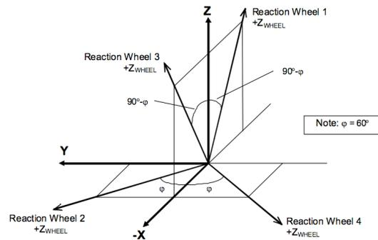
Figure 2. Reaction wheels spin axes orientation.
