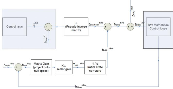
Figure 4. Control Block Diagram of the 4WD design.
