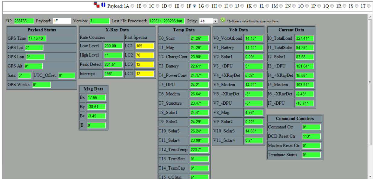
Figure 4. Live Data Viewer. The Live Data Viewer gives a quick way to see all data that are transmitted from the payload. These data are checked against threshold values and will change color if out of range.
