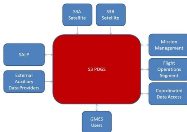
**Figure 1. Sentinel-3 PDGS External Interfaces.**
