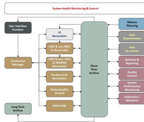
**Figure 5. PDGS Functions at Marine Center.**
