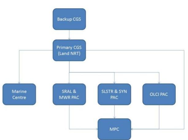
**Figure 3. Sentinel-3 PDGS Centers.** The diagram depicts the center layout and the main data flows.
