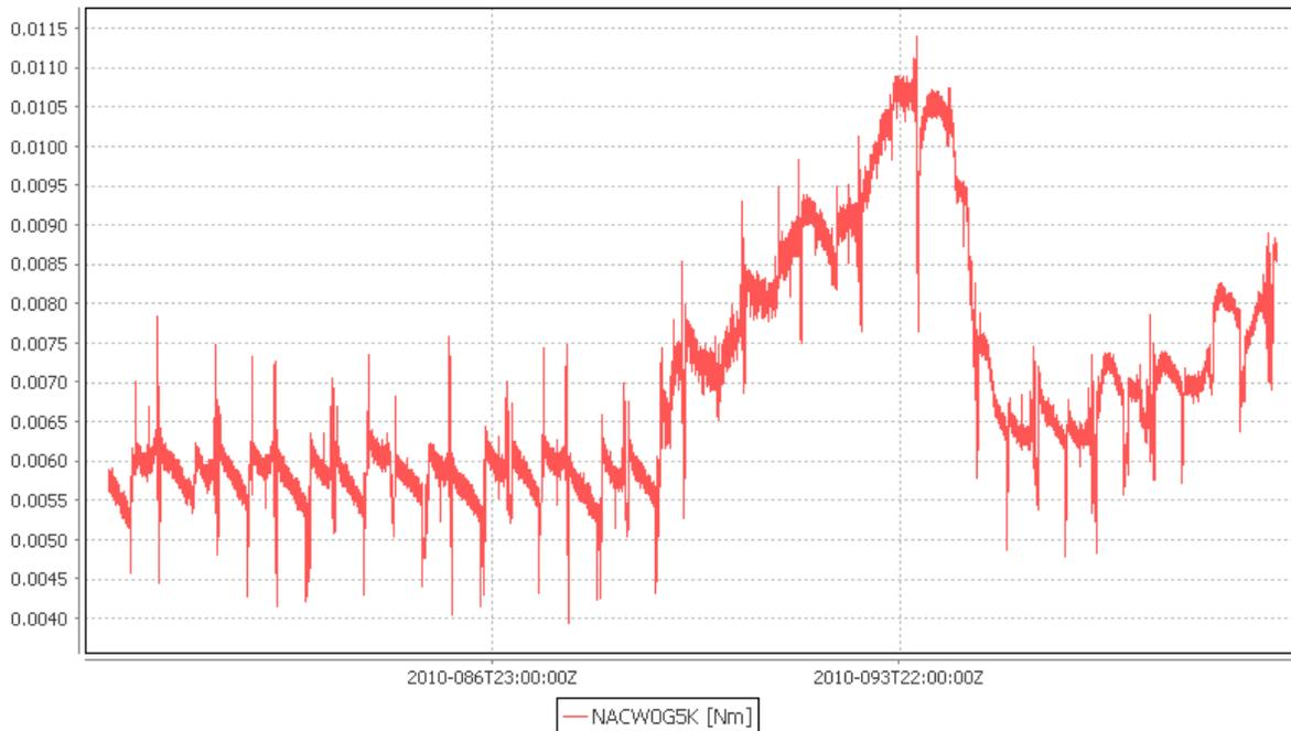
**Figure 1. Venus Express Reaction Wheel 4 Friction increases starting in Day of Year 2010.89.** *This behavior was not detected by Out-Of-Limits alerts as the upper limit was set to 0.02 at that time. In this case, this behavior was recognized by Venus Express engineers as they closely monitor the reaction wheels even if they do not trigger any Out-Of-Limits.*
