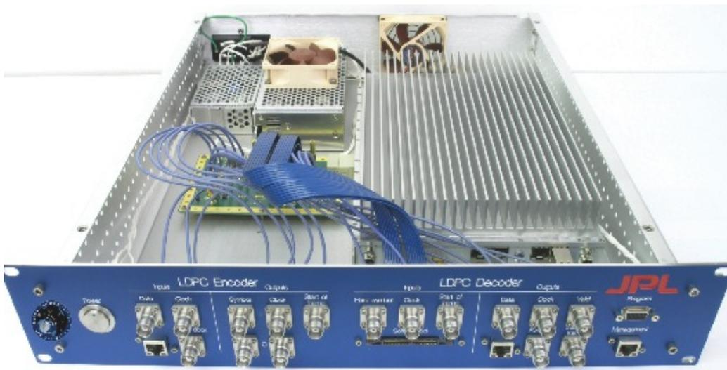
Figure 3. SCaN Baseband Emulator and LDPC Codec
