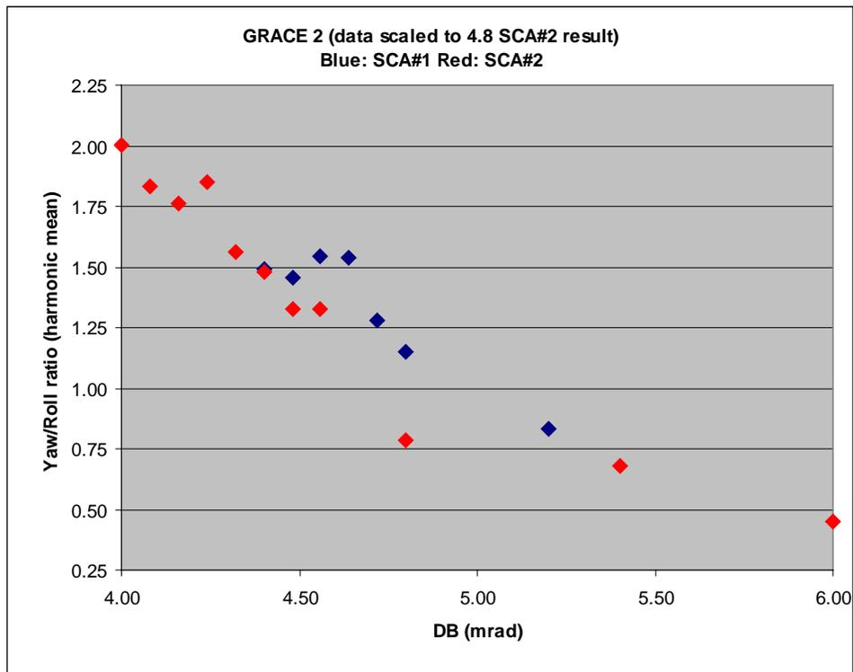
Figure 7. The ratio of yaw over roll thruster actuations as a function of yaw dead band. Each point represents the results of a seven day campaign. Data measured with different star cameras as prime have been scaled to fit (see text for full details).
