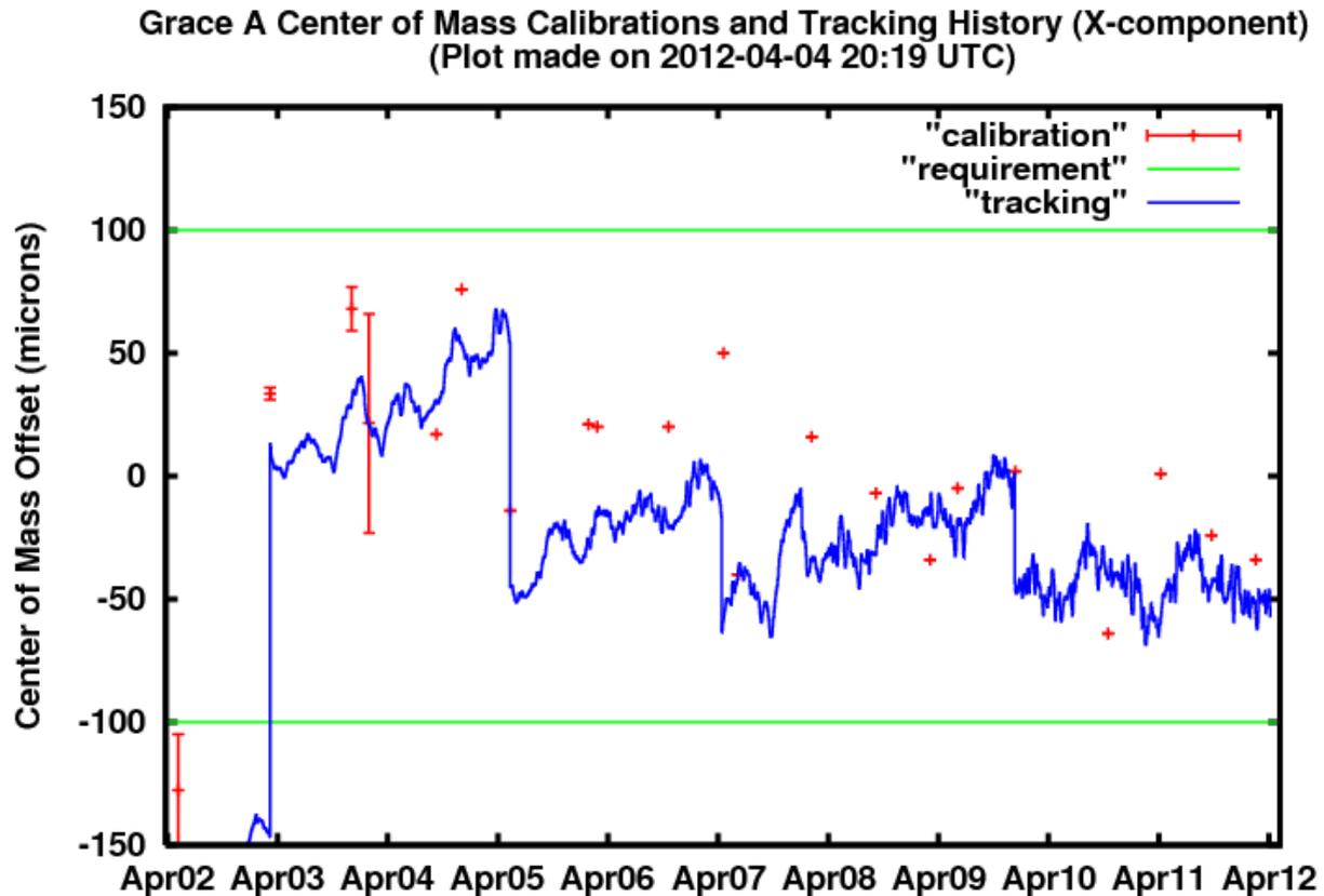
**Figure 6. Results of the CoM calibrations in the roll axis.** *The in-orbit measurements (red symbols) are compared with a tracking model based upon the differential depletion of the two fuel tanks (JPL website for GRACE monitoring).*
