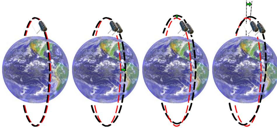
**Figure 2. Formation building with relative eccentricity / inclination vector separation.** *From left to right: (1) identical orbits, (2) horizontal separation at equator crossings by small offset in the ascending node (green arrow indicates RAAN offset), (3) small eccentricity offset causes different heights of perigee / apogee and hence yields radial separation at poles. (4) Optional rotation of the argument of perigee to achieve larger baselines at high latitude regions.*
