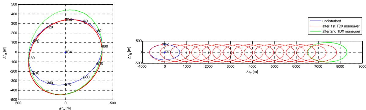
**Figure 9. Illustration of formation breakup scenario.** *TDX performs an orbit lowering maneuver at north polar crossing (transition from blue to red relative motion ellipse). The initialized along-track drift is depicted right. After 1 day a second maneuver is performed to stop the drift at 7.5 km mean along-track distance from TSX (green ellipse).*
