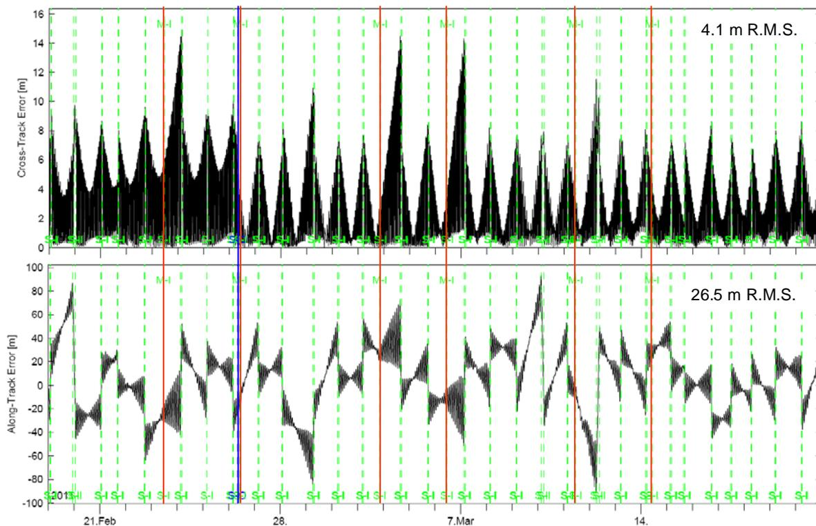
**Figure 4. Formation control performance (Feb. 19 to Mar. 21, 2011).** Top: the combined radial and normal error (i.e. cross-track error, 2D) is 4.1 m R.M.S. (requirement: 28.3 m). Bottom: the along-track error amounts to 26.5 m R.M.S. (requirement: 200 m). The vertical lines indicate common TSX/TDX maneuvers (red) and TDX formation maintenance maneuvers (green: in-plane, blue: out-of-plane).
