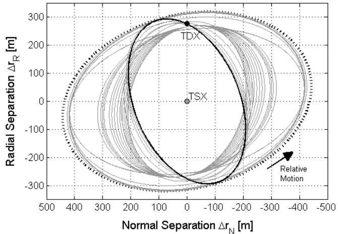
**Figure 6. Evolution of TDX-TSX relative motion during the period from Dec. 2010 (dotted ellipse) to Dec. 2011 (bold black ellipse).** The relative motion is shown in the plane perpendicular to flight direction. The filled black circle indicates the TDX relative position at 90 deg argument of latitude (north polar crossing).
