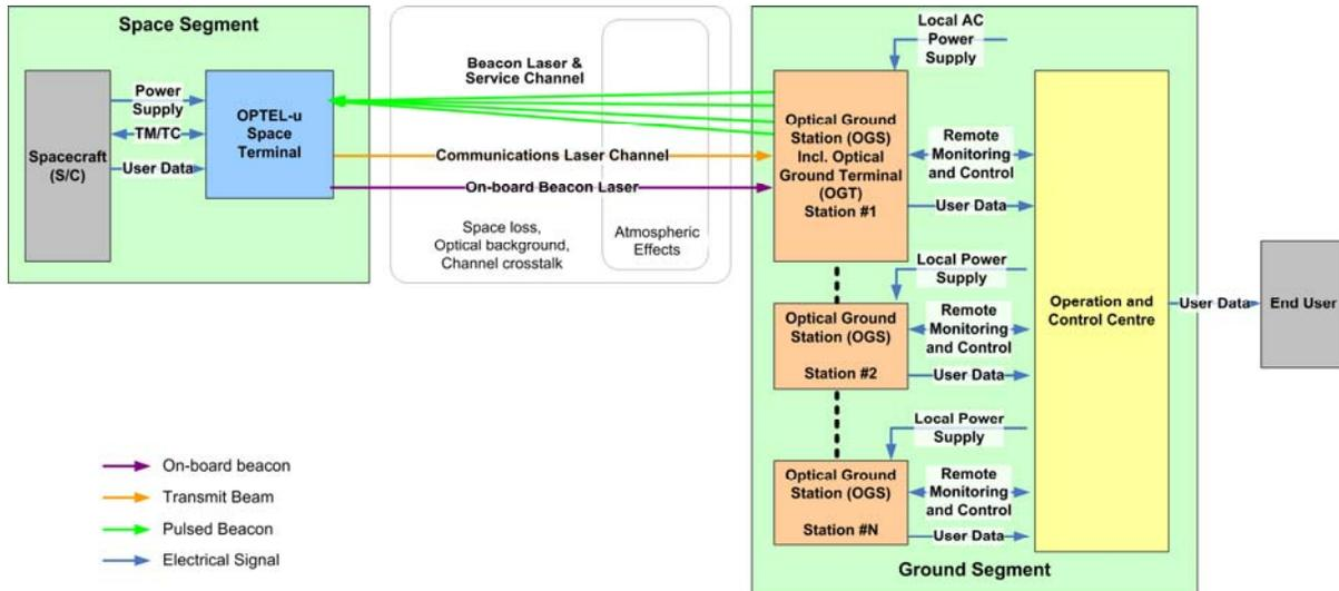
Figure 1. OPTEL  $\mu$  system Block diagram.
