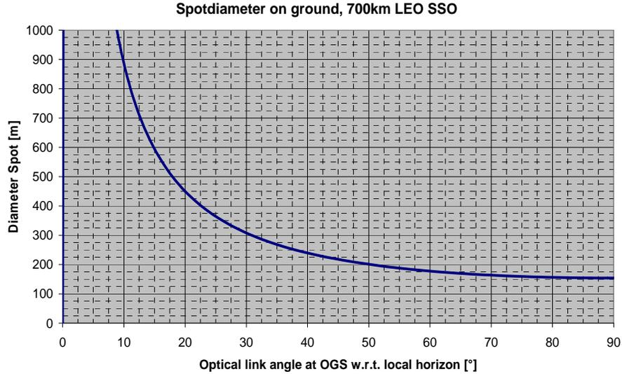
**Figure 5. OPTEL- $\mu$  spot diameter as function of ground elevation angle.**
