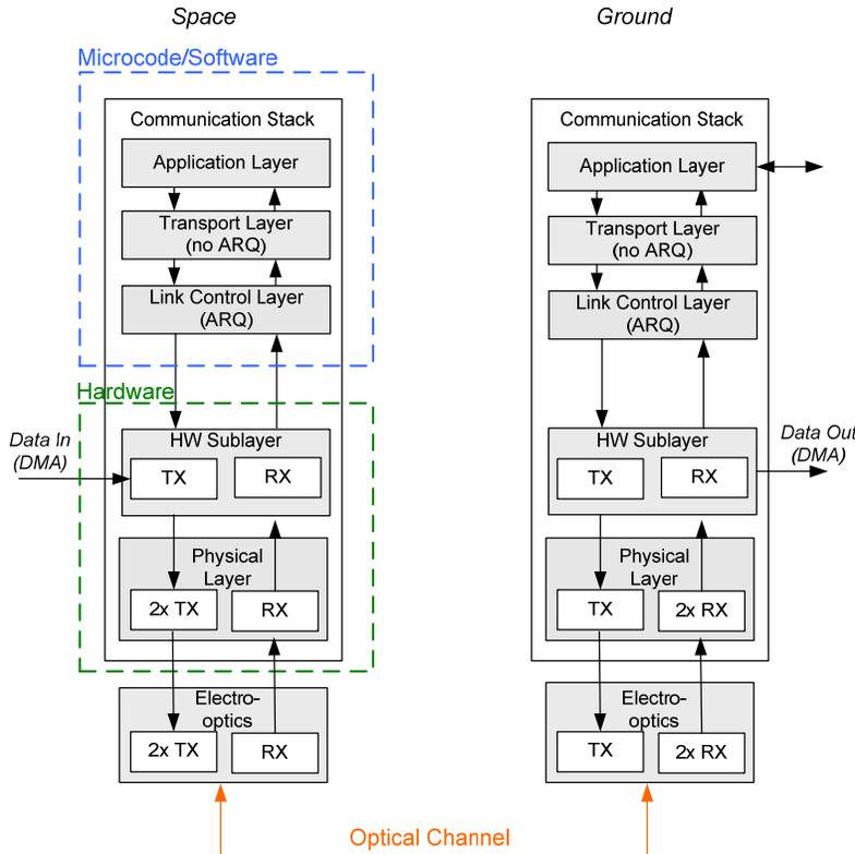
Figure 7. Block diagram OPTEL- $\mu$  Link Layer Architecture
