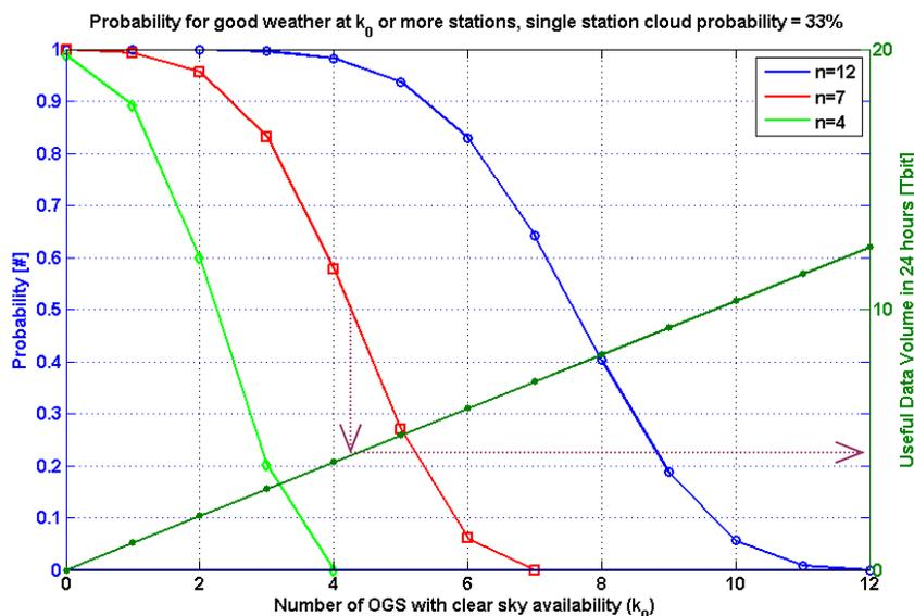
**Figure 3. Binominal Distribution Model for prediction of downlink volume from one Space Terminal.** Contact times use simulated downlink passages for a strawman mission in 700km SSO. Downlink data rates are extrapolated based on accredited link budget formula, using receiver sensitivity data measured at RUAG.
