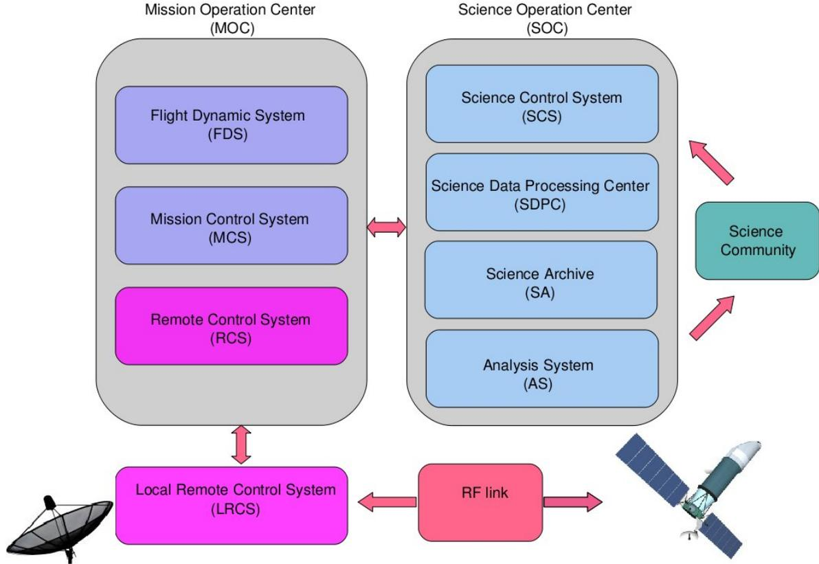
Figure 2: Layout of the WSO-UV Ground Segment
