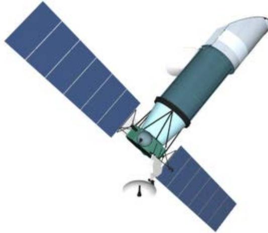
Figure 1: The WSO-UV Space telescope
