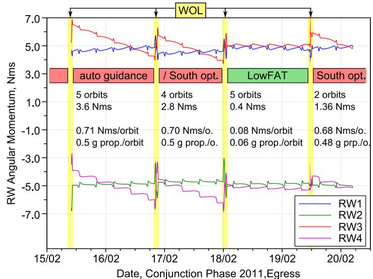
**Figure 4. Reaction wheel levels during LowFAT test from s/c telemetry.** For periods between wheel off-loadings additional information is displayed: number of orbits, total angular momentum build-up, build-up per orbit and propellant required per orbit. In LowFAT the build-up of angular momentum is significantly smaller than in the adjacent auto guidance phases.
