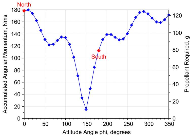
Figure 2. Angular momentum accumulated at different values of the angle phi. Calculated for the conjunction period from 17/01 to 20/02/2011. The scale on the right shows the amount of propellant necessary to neutralize the accumulated angular momentum.
