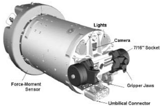
**Figure 3. ORU/Tool Changeout Mechanism**
