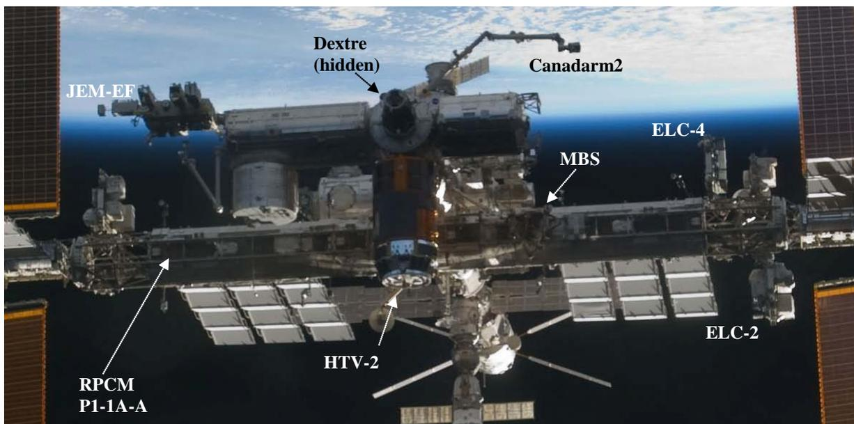
**Figure 5. Dextre Work Areas on ISS for 2011**
