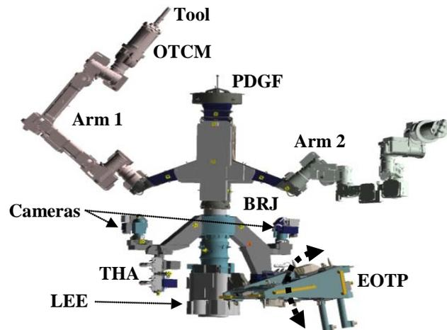
Figure 2. Dextre Components
