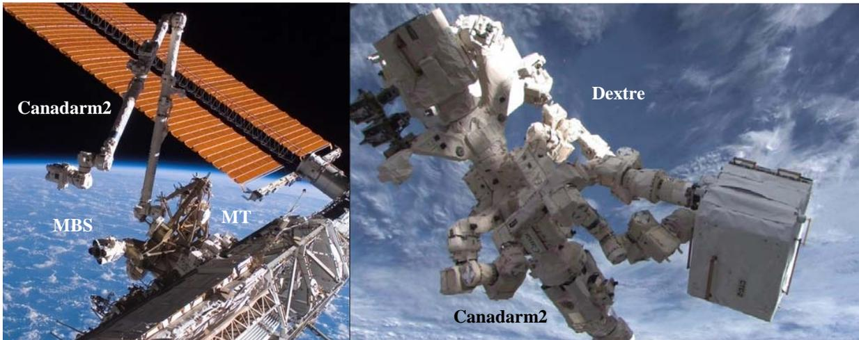
Figure 1. The Mobile Servicing System
