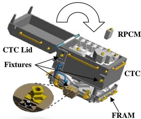
**Figure 4. Dextre-Compatible Cargo Transport Container and Flight Releaseable Attach Mechanism**
