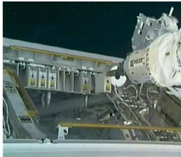
**Figure 11. Dextre Extracting Failed RPCM from P1-1A-A Site**
