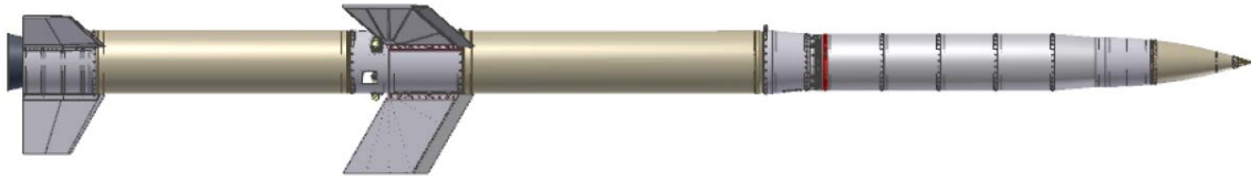
Figure 9. MAIUS-1 Vehicle consisting of a VSB-30 rocket motor assembly and payload.
