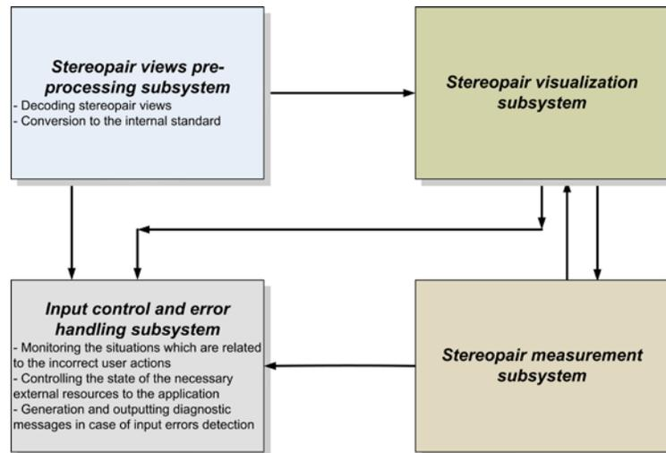
**Figure 1 The functional scheme of the digital stereo comparator**
