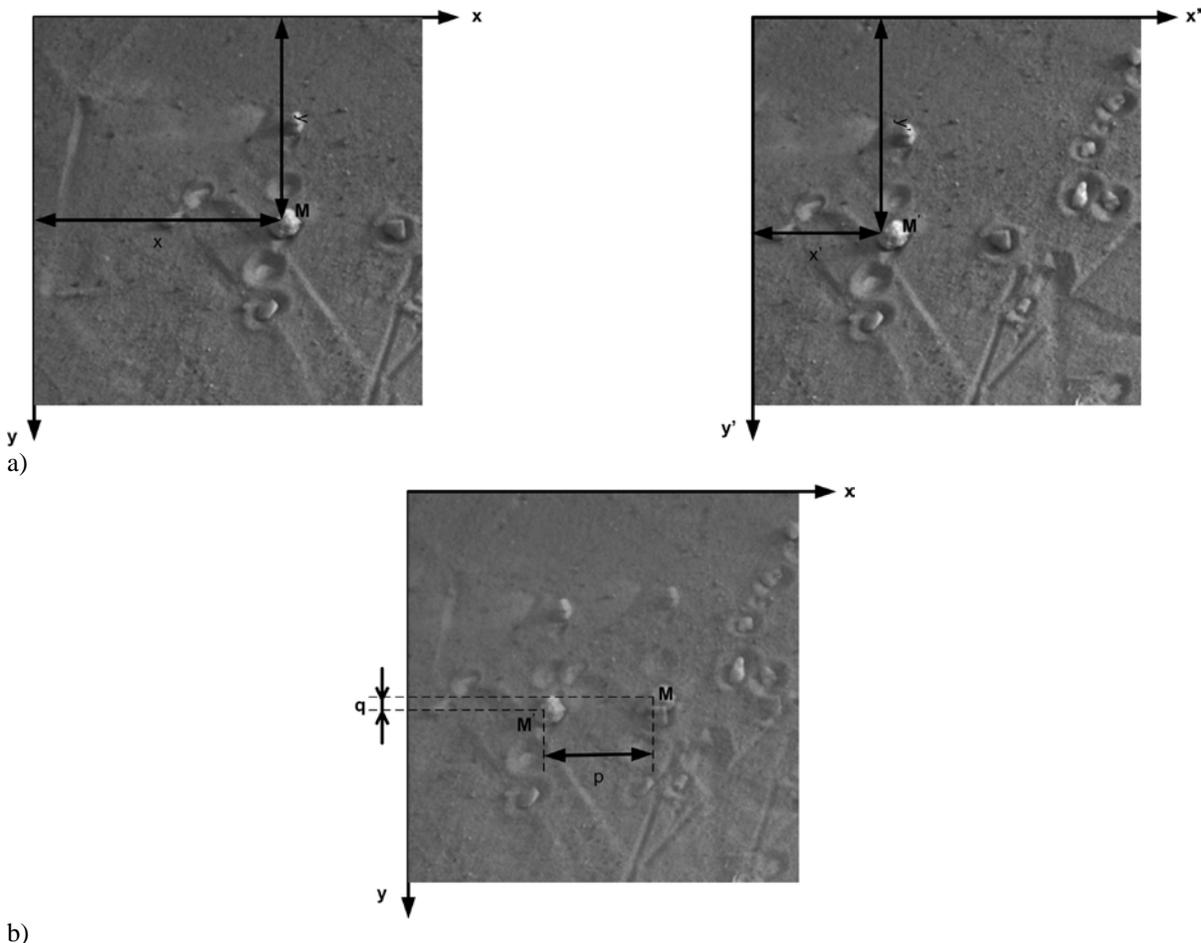
**Figure 4 The principle of stereo measurements**
