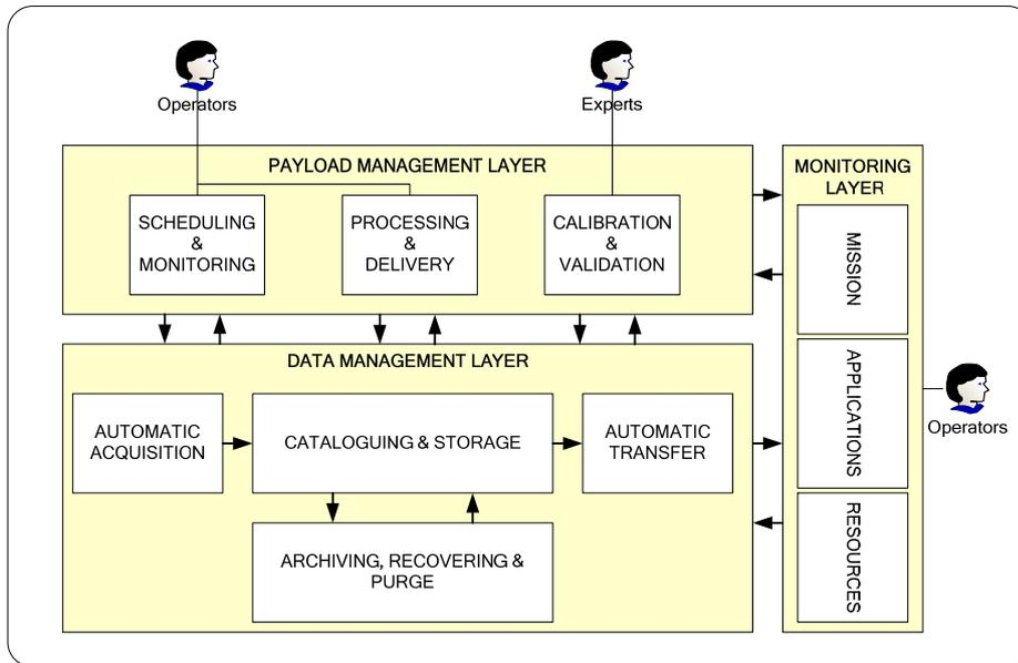
**Figure 1. Functional architecture of a payload ground system**
