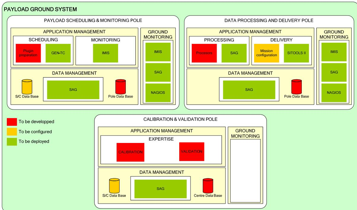
**Figure 3. Software and functional architecture of a reusable payload ground segment.**
