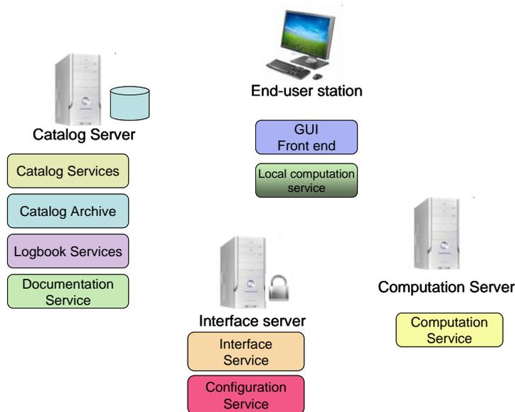
**Figure 4. SAG Service Oriented Architecture**
