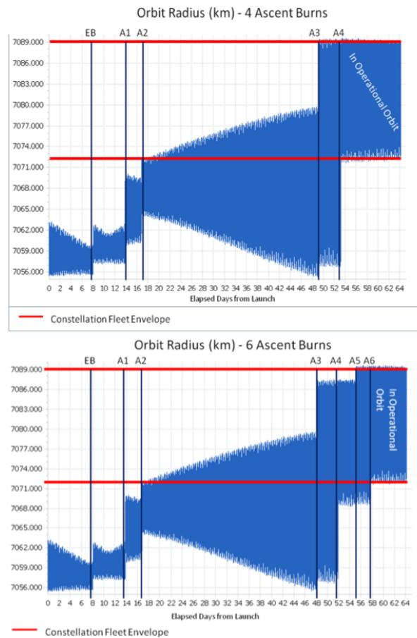
**Figure 2. LDCM Orbit Radius History for a 4-burn ascent (Top) and a 6-burn ascent (Bottom) with respect to the constellation fleet envelope (shown in red).**
