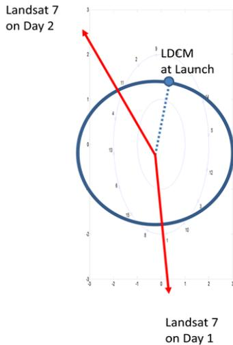
**Figure 4. LDCM-Landsat 7 relative phasing for each day of the 16-day cycle at the beginning of the launch time window.**
