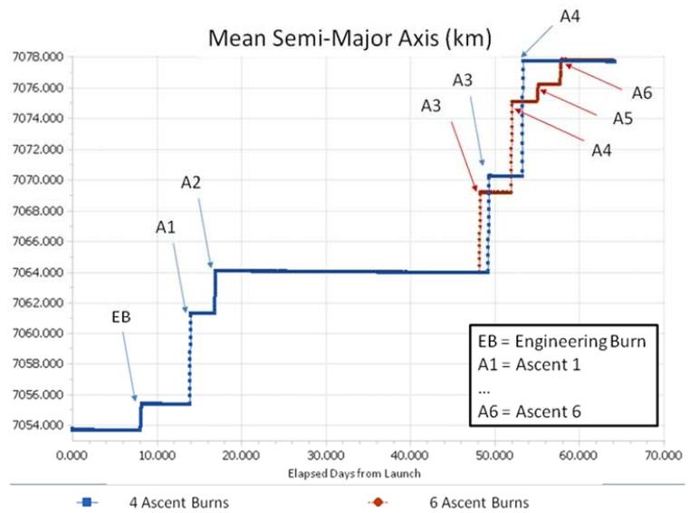
**Figure 1. Mean Semi-Major Axis Evolution for a 6 ascent burns versus a 4 ascent burns scenario.**
