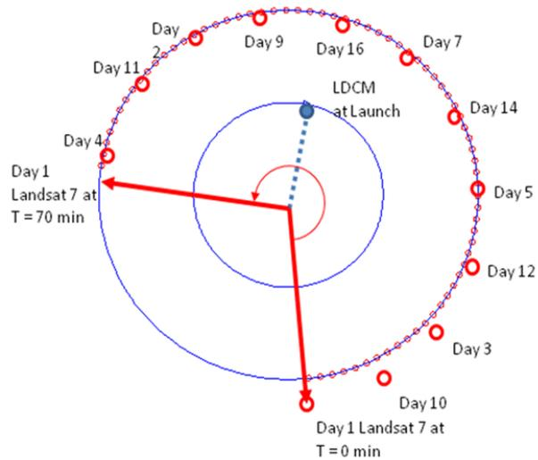
**Figure 5. LDCM-Landsat 7 relative phasing for Day 1 for the entire launch time window**
