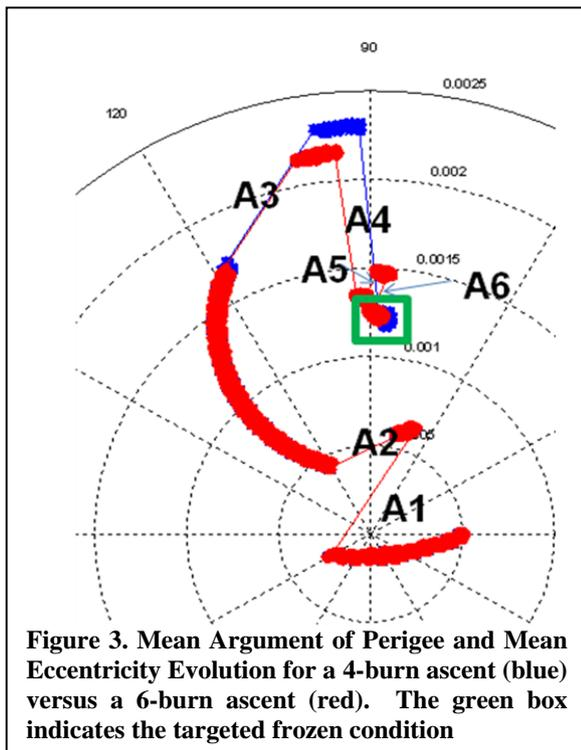
**Figure 3. Mean Argument of Perigee and Mean Eccentricity Evolution for a 4-burn ascent (blue) versus a 6-burn ascent (red). The green box indicates the targeted frozen condition**
