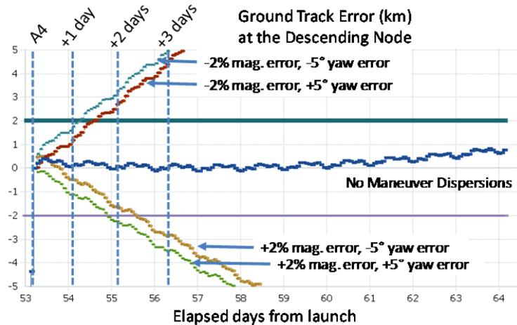
**Figure 7. Ground Track Error (km) History for Different Maneuver Execution Errors for Ascent 4 Burn.**
