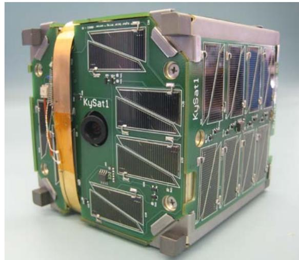
**Figure 1. KySat-2 CubeSat Under Development is an Updated Version of KySat-1 (shown above) that was lost during a failed launch attempt on a Taurus A from Vandenberg Air Force Base in 2011**
