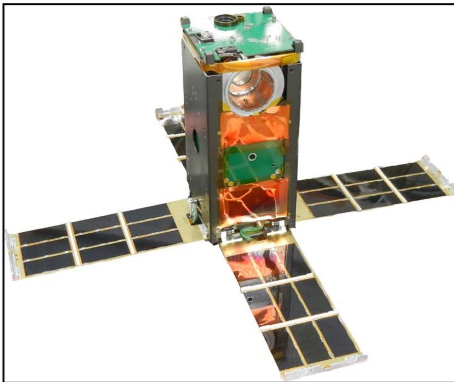
**Figure 2.** *Cosmic X-Ray Background NanoSatellite (CXBN) was developed in 2011 by the Space Science Center at Morehead State University. CXBN is scheduled for launch in August 2012 and will measure the diffuse X-ray background emission from the Big Bang.*
