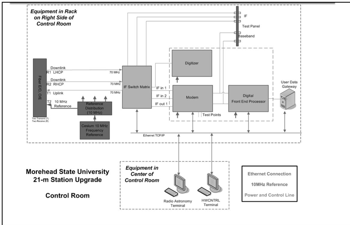
Figure 6. Block Diagram of the 21-m Digital Signal Processing Architecture
