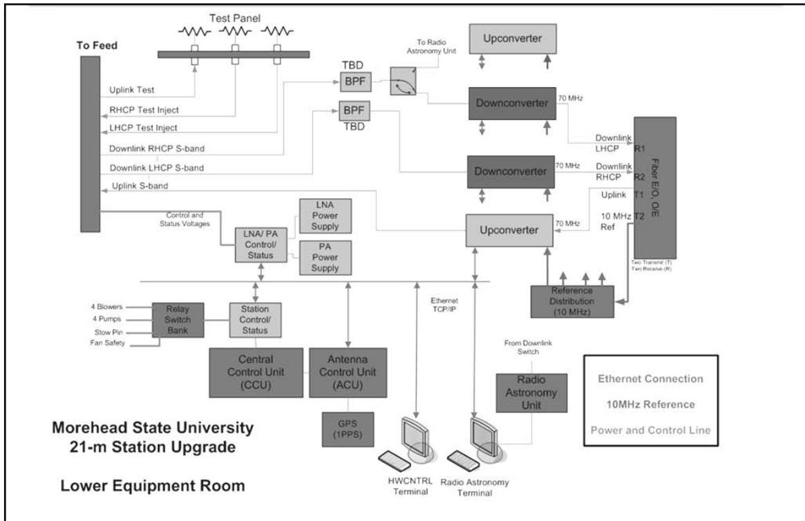
Figure 7. Block Diagram of the 21-m IF, Front-end Processor and Remote Operations Architecture
