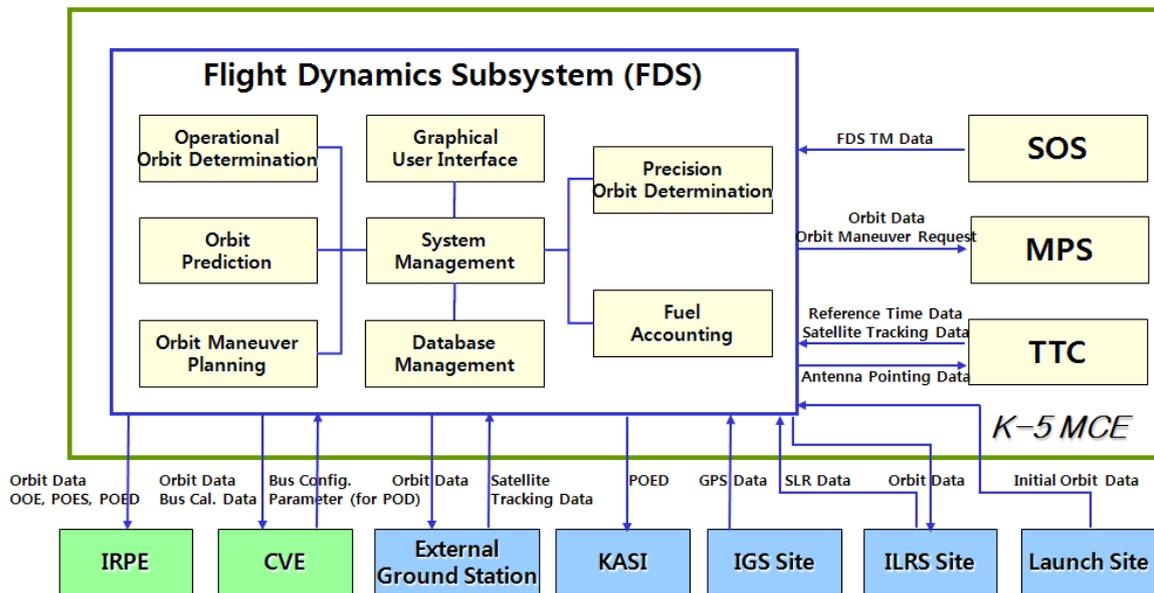
Figure 4. Functional Architecture and Internal/External Interface of FDS
