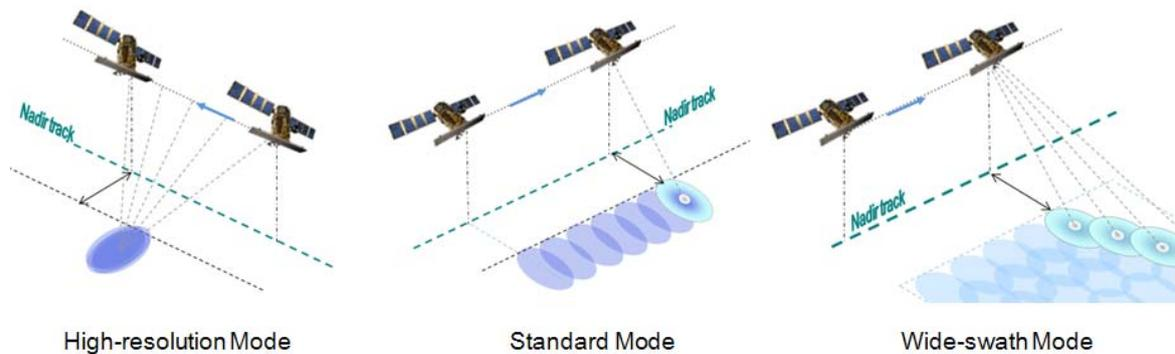
**Figure 2. Multiple Imaging Modes of KOMPSAT-5 SAR Operation**
