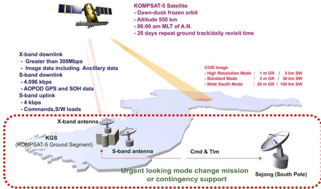
Figure 3. System Architecture of KOMPSAT-5
