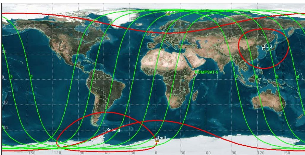
**Figure 5. Expected Initial Ground Track of KOMPSAT-5 (Starting from Separation Point)**
