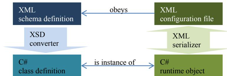
**Figure 1. Interaction in between schema and code**
